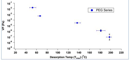
Figure 4: Reported vapour pressure measurements of the PEG series (4-8) and associated  $T_{max}$  values extracted from the UMan FIGAERO-CIMS. Errors on the y-axis are those reported in the Kreiger et al., (2018) study. Errors in the  $T_{max}$  (x-axis) are the maximum variation seen within the 4 thermograms from which the mean value was derived.
