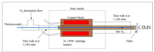
Figure 2: internal schematic of the FIGAERO desorption gas heater unit. Temperature above the filter is measured at the end point of the heated tube by the long thermocouple running through the inlet, shown here in blue.
