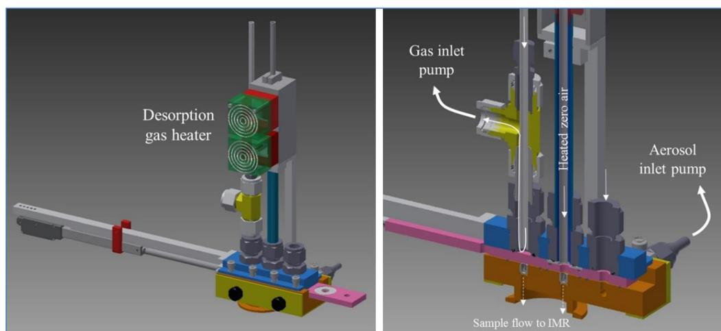
30 **Figure 1: Drawing of the ARI FIGAERO assembly. Panel on left shows full assembly with mechanical actuator that controls gas sampling/aerosol collection or aerosol desorption operating modes. Panel on right is a cross-sectional view that show flows for both gas and particle sampling mode and the two apertures that connect with the IMR. In this view the FIGAERO slide is positioned in the aerosol desorption mode and the gas sample flow into the IMR is closed.**
