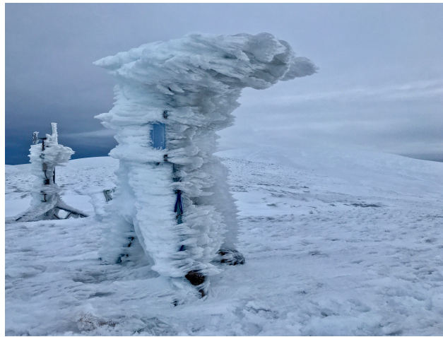
Figure 6. Disdrometer at Druim nam Bo, Scotland covered in rime in January 2018. The instrument was still receiving power and recording nullified (no beam received by optical diode) data which it interpreted as a 'sensor error' (-1) present weather code.
