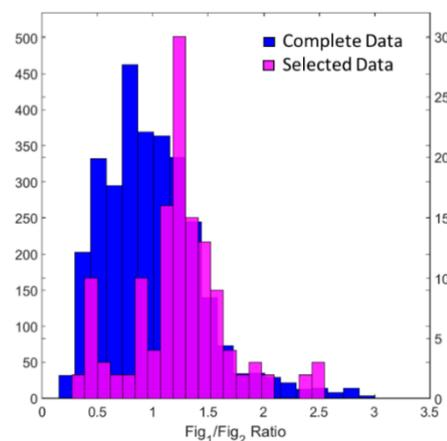
**Figure 11:** Histogram of complete sensor ratios for each hour using moving correlation window vs. the ratios for a select subset of data with high correlation between benzene and methane ( $> 0.85$ ), a ratio of benzene:methane typically associated with oil and gas activity ( $< 1.0$  ppb/ppm), and a significant change in methane ( $> 0.5$  ppm).
