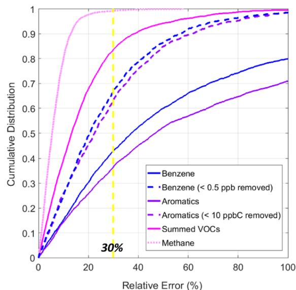
**Figure 6: Cumulative distributions of relative sensor error for all fitted testing or validation data, the two dotted lines represent the fitted testing data for benzene and summed aromatic, respectively, with the low values removed from the reference data.**
