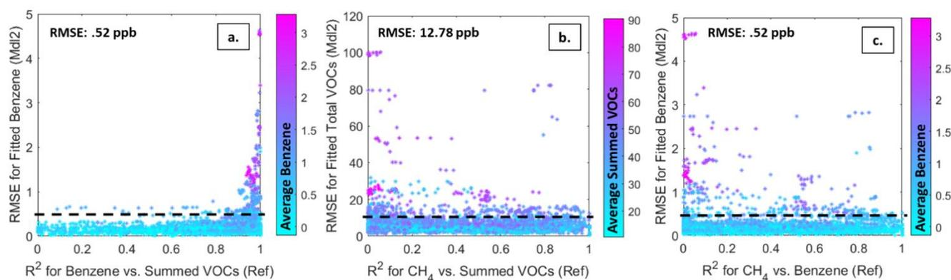
**Figure 8: Plots of error (RMSE) versus the coefficient of determination ( $R^2$ ) for the target VOC or group versus a non-target, potentially confounding VOC or group. These values are calculated on the basis of a 1-hour moving window and the points are colored according to the average of the target pollutant or group for that hour. The dotted black line on each is the overall RMSE determined in Section 3.1.**
