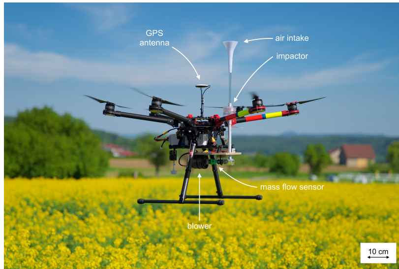
Figure 1. Multicopter UAV (DJI S900) in hovering flight with components of the particle collection system as indicated: air intake, impactor, mass flow sensor, and blower. The inlet of the air intake is arranged about 30 cm above the propeller plane.
