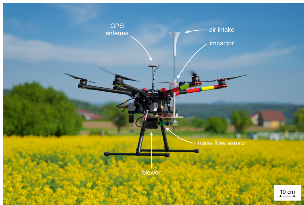
Figure 1. Multicopter UAV (DJI S900) in hovering flight with components of the particle collection system as indicated: air intake, impactor, mass flow sensor, and blower. The inlet of the air intake is arranged about 30 cm above the propeller plane.
