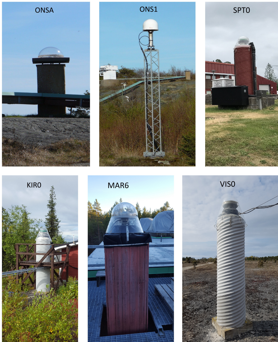
Figure 3. The six antenna installations used to acquire the GPS data. See Figure 2 for their geographical location.
