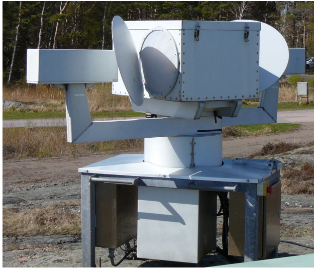
Figure 4. The water vapour radiometer (WVR) Konrad at the Onsala Space Observatory.
