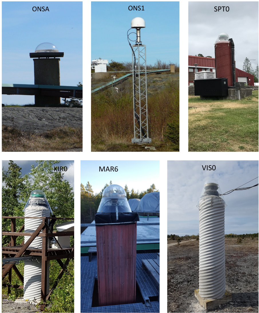
Figure 2. The six antenna installations used to acquire the GPS data. See Figure 1 for their geographical location.
