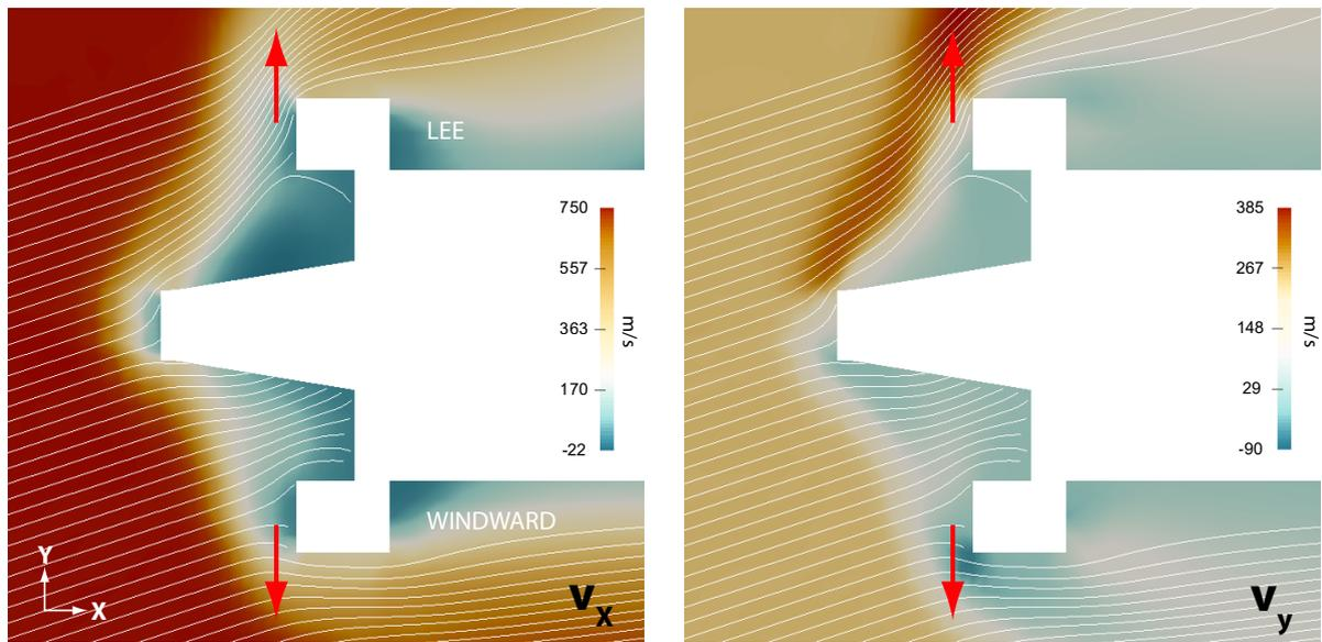
**Figure 9.** Numerical results of an aerodynamic simulation of the payload at a trajectory point in 85 km altitude during downleg. Colors indicate the components of the velocity vector. *Left:* longitudinal ( $x$ ), *right:* lateral ( $y$ ). Red arrows mark the sensor position and the orientation of the electrode surface.
