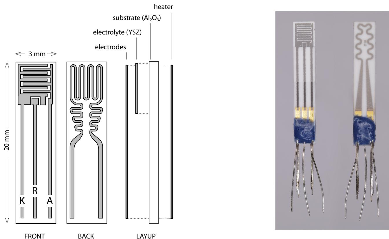
**Figure 1.** *Left:* schematic layout of the 3-electrode FIPEX sensors. Front side with interdigitated electrodes, back side with resistance heater. *Right:* Photo of a screen printed sensor with platinum electrodes. The leads are sealed with a blue glass layer.
