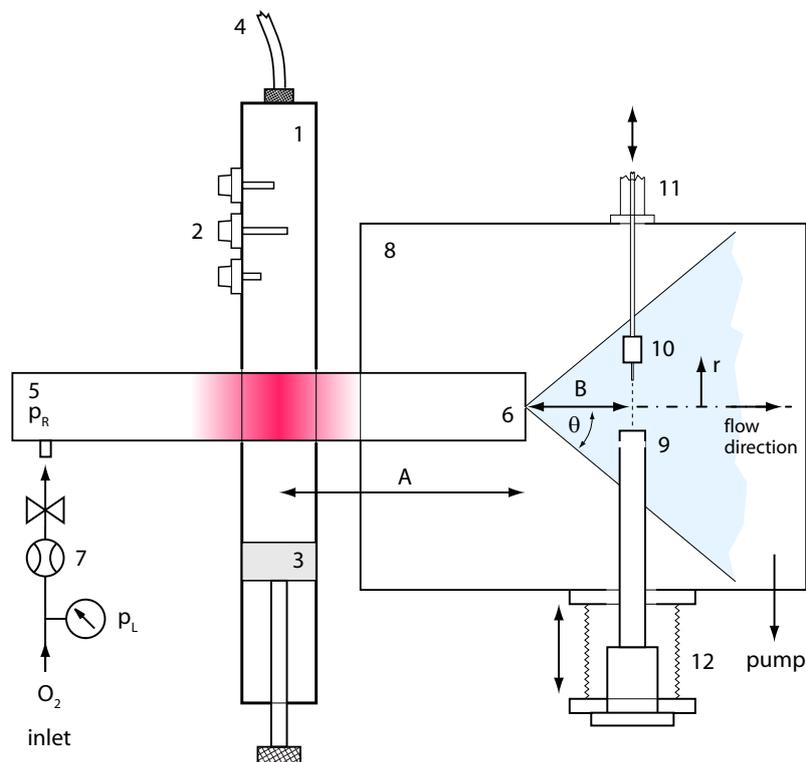
**Figure 3.** Calibration setup for atomic oxygen. 1 - microwave wave guide, 2/3 tuner and short circuit for impedance matching, 4 - coaxial line, 5 - fused silica tube, 6 - orifice, 7 - O<sub>2</sub>-inlet with bubble flowmeter, 8 - high vacuum chamber, 9 - mass spectrometer with cross-beam ion source, 10 - solid electrolyte sensor in mounting, 11 - moveable vacuum manipulator, 12 - movable bellows.
