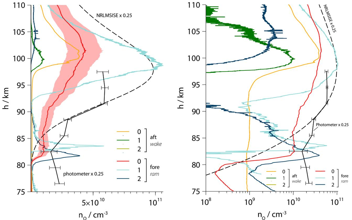
**Figure 11.** *Left:* Vertical profile of the atomic oxygen number density along the upleg of WADIS-2 including aerodynamic corrections. Fore sensors are in ram, aft sensors in wake. Values of Aft-2 are all zero. The shading around the profile of sensor Fore-0 indicates the uncertainty of the calibration. The scaled profiles derived from the on-board airglow photometer data and the NRLMSISE-00 atmospheric model are sketched for comparison. *Right:* Semi-logarithmic plotting.
