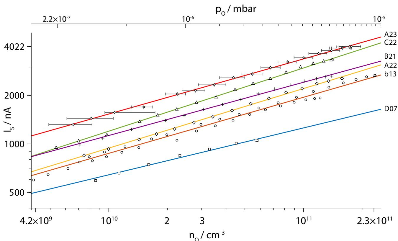
**Figure 5.** Calibration curves for atomic oxygen for sensors used on the WADIS-2 campaign in double-logarithmic plotting for a reference temperature of 293 K. Solid lines represent power functions fitted to the measurement data. The uncertainty of the calibration is given exemplarily for sensor A23, with the standard deviation of  $I_s$  below 10 nA.
