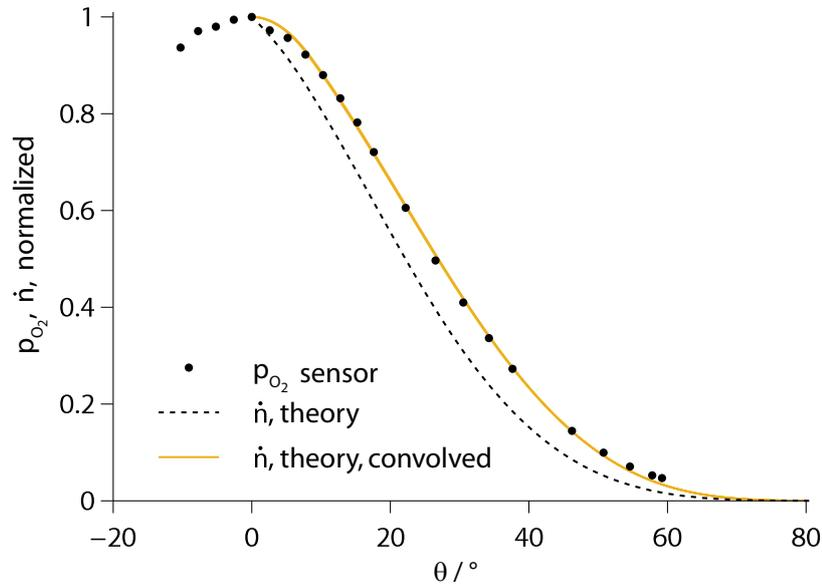
**Figure 4.** Theoretical profile of the number flux density according to Giordmaine et al. (Giordmaine and Wang, 1960), convolved with the electrode length and fitted to the measurement data of a platinum sensor (solid line). The profile prior to convolution is given additionally (broken line).
