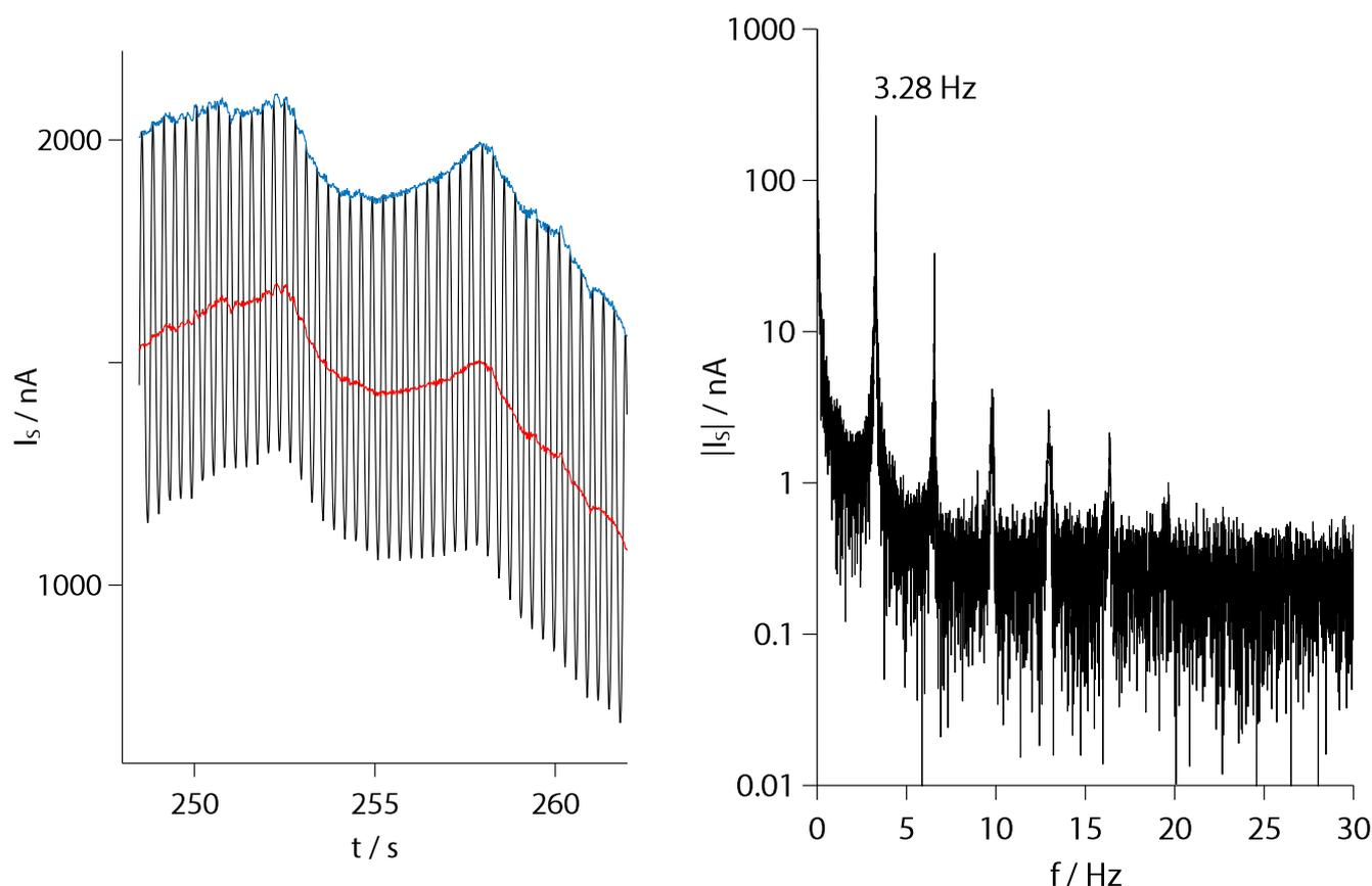
**Figure 10.** *Left:* Detail of the transient sensor signal showing periodical oscillations due to the payload rotation. The red curve is the result of a filtering by several narrow-bandwidth notch filters, the blue curve is obtained by subsequent fitting to the maximums. *Right:* Frequency spectrum of the raw signal with clear peaks at the rotational frequency and its harmonics.
