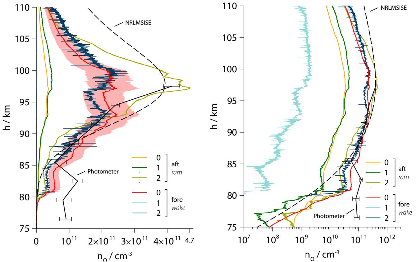
**Figure 12.** *Left:* Vertical profile of the atomic oxygen number density along the downleg of WADIS-2 including aerodynamic corrections. Aft sensors are in ram, fore sensors in wake. Values of Aft-2 are all zero. The shading around the profile of sensor Fore-0 indicates the uncertainty of the calibration. The profiles derived from the on-board airglow photometer data and the NRLMSISE-00 atmospheric model are sketched for comparison. *Right:* Half-logarithmic plotting.
