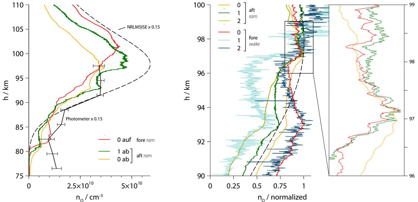
**Figure 13.** *Left:* Comparison of the ram-profiles of different sensors, measured by Fore-0 during the upleg as well as by Aft-0 and Aft-1 during the downleg. Profile derived from the photometer data and values of the NRLMSISE-00 atmospheric model are scaled by a factor of 0.15. *Right:* Normalized profiles of all sensors during the downleg, with fore sensors in wake- and aft sensors in ram position. The inset shows a detail of the profiles featuring small scale variations.
