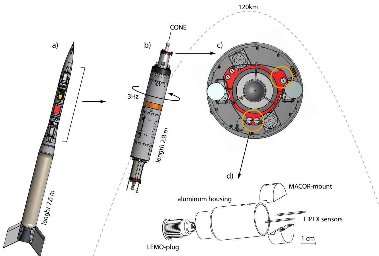
**Figure 6.** Rocket configuration of the WADIS mission. a) Total view including motor and nose cone. b) Spin-stabilized payload with instrument decks on fore and aft and sketched trajectory. c) Details of the fore deck with highlighted positions of the FIPEX sensor heads. d) Assembly of a sensor head with two sensors mounted in an aluminum housing.
