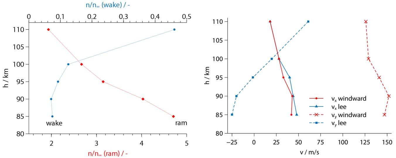
**Figure 8.** *Left:* Aerodynamic correction factors for sensors in *ram* and *wake* position derived from numerical simulations at the windward side. Each dot represents a calculated trajectory point. *Right:* Longitudinal ( $x$ ) and lateral ( $y$ ) velocity components at the sensor position, calculated in *ram*.
