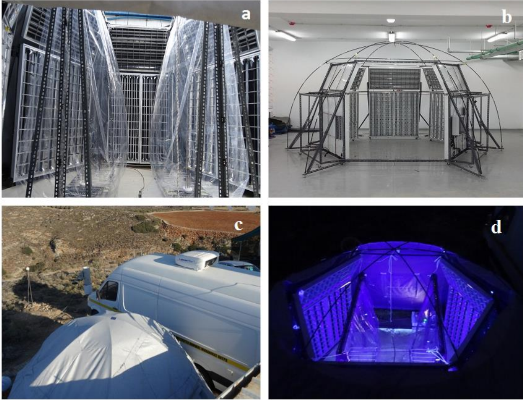
Figure 1. Pictures of the portable dual chamber system: a) the dual chambers; b) UV light assembly; c) field deployment during the FAME 16 study; d) system configuration with the UV lights on and the top cover open.
