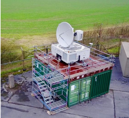
95 Figure 3. NXPol deployed at Chilbolton Observatory, Hampshire, UK. Seen in the picture is the 20' shipping container, 20' office 96 container, two 20' platform containers and scaffolding used to construct a platform for the radar.
