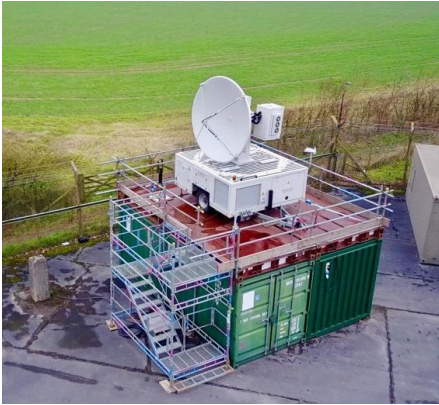
75 Figure 3. NXPol deployed at Chilbolton Observatory, Hampshire, UK. Seen in the picture is the 20' shipping container, 20' office 76 container, two 20' platform containers and scaffolding used to construct a platform for the radar.
