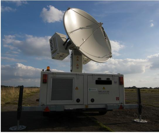
Figure 1: Photograph of the NXPol collecting data at Burn Airfield near Selby, UK. Here the NXPol is deployed using only its 52
