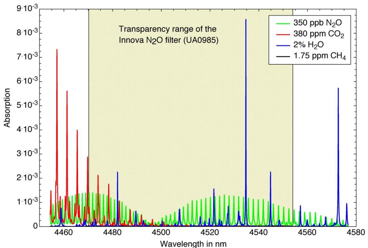
Figure 1: Broadband filters used within the Innova family. As an example, the  $N_2O$  transparency window includes absorption bands for  $CO_2$  and  $H_2O$ .
