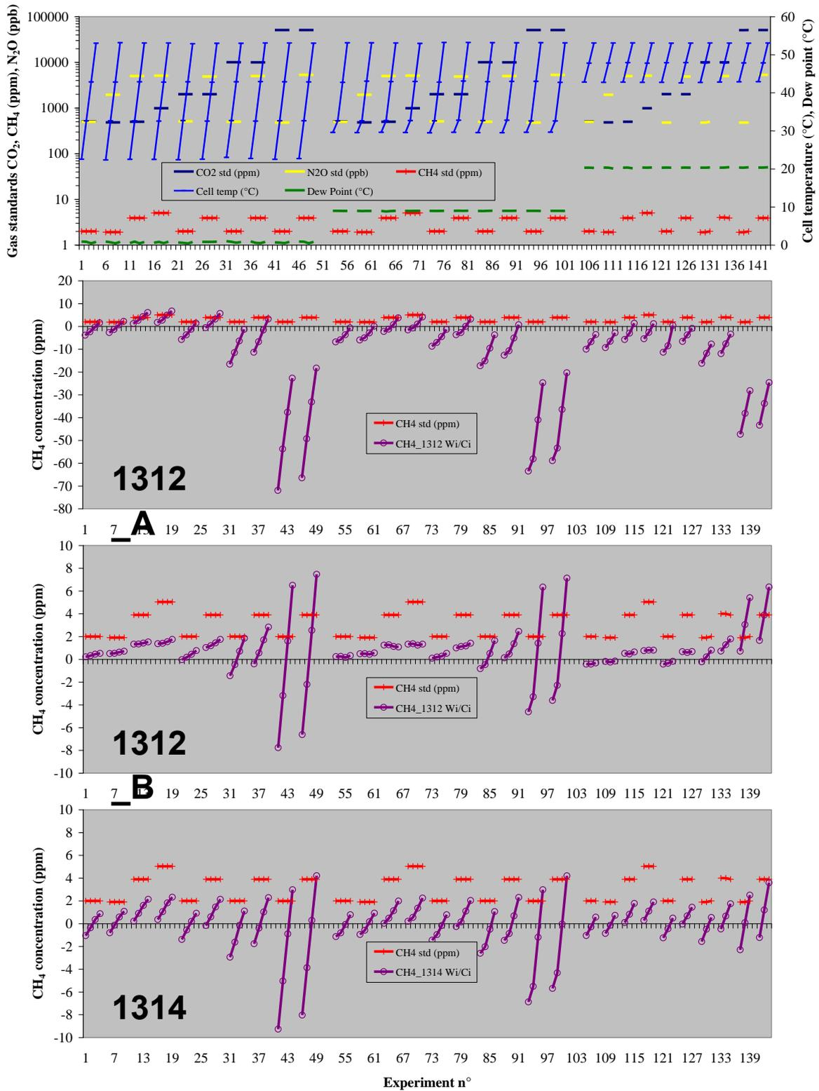
Figure 3c CH<sub>4</sub> concentration determined by the Innova's instruments. The number on the x-axis refers to trials with conditions as given in the first panel. The solid lines in the panels indicates the applied standard gas concentration for CH<sub>4</sub>.
