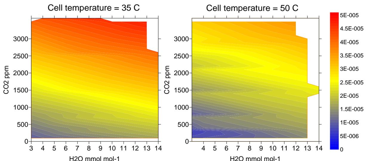
Figure 2 shows the effect of varying CO<sub>2</sub> and H<sub>2</sub>O concentrations on the raw signal strength of the N<sub>2</sub>O filter UA0985
