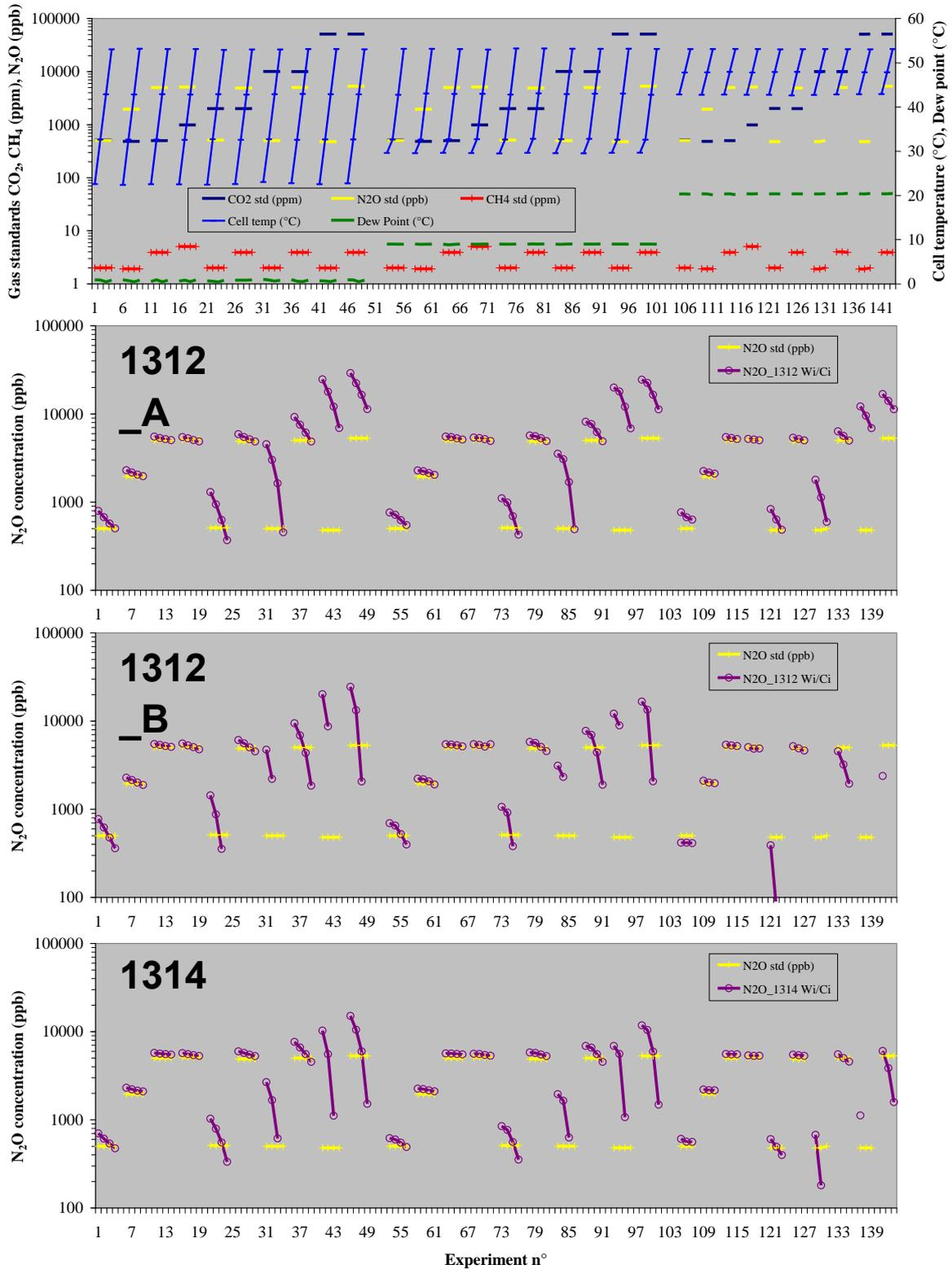
Figure 3b N<sub>2</sub>O concentration determined by the Innova's instruments. The number on the x-axis refers to trials with conditions as given in the first panel. The solid lines in the panels indicates the applied standard gas concentration for N<sub>2</sub>O
