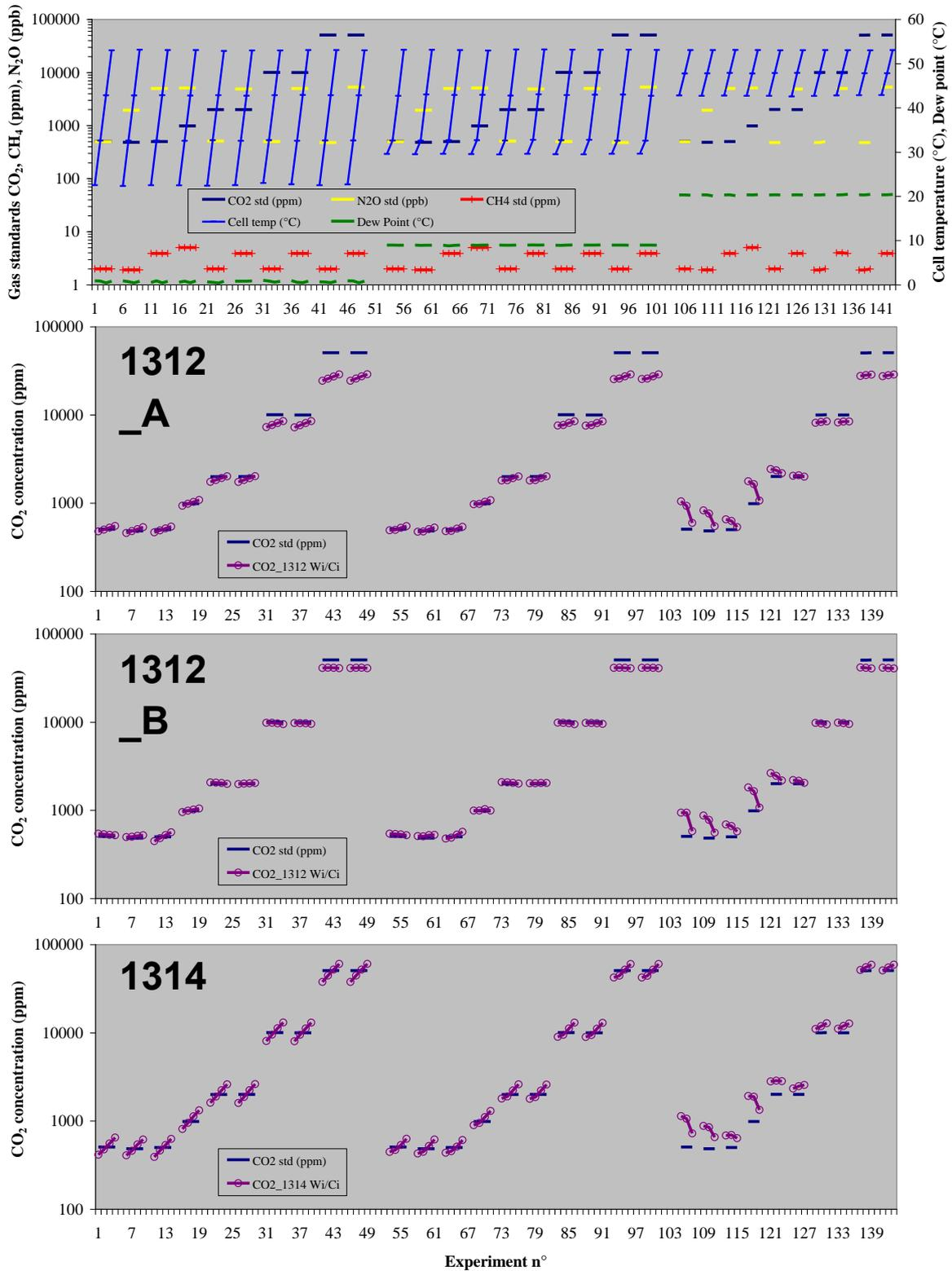
Figure 3a CO<sub>2</sub> concentration determined by the Innova's instruments. The number on the x-axis refers to trials with conditions as given in the first panel. The solid lines in the panels indicates the applied standard gas concentration for CO<sub>2</sub>.
