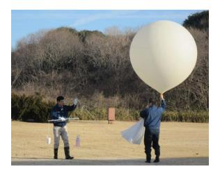
Figure S1: Preparations for a flight launch at 8:30 local time on January 6, 2017. RS-11G and RS92 units were hung on the ends of a plastic/cardboard rod.
