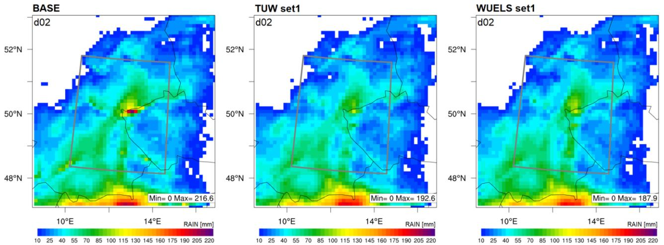
**Figure 12: Total precipitation accumulated for 72 hours (2013-05-31 00 UTC - 2013-06-03 00 UTC) for the WRF model forecasts: BASE (left), TUW set1 (middle), and WUELS set1 (right). The grey line indicates the boundaries of the GNSS tomography models' inner domain.**
