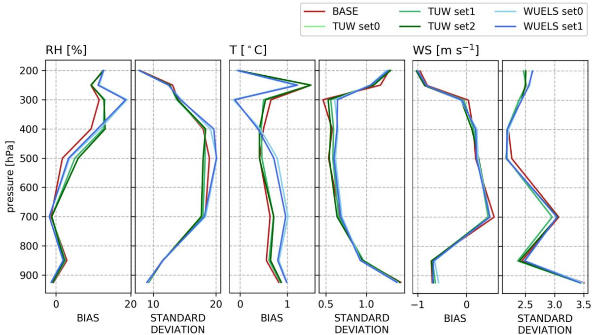
5 **Figure 13: From the right, statistics (bias, standard deviation) for Relative Humidity (RH), Temperature (T), and Wind Speed (WS) base forecast and model fed with TUW (set0, set1, set2) and WUELS (set0, set1) data when compared with radiosonde measurement; comparison at assimilation time (6 hours since model start).**
