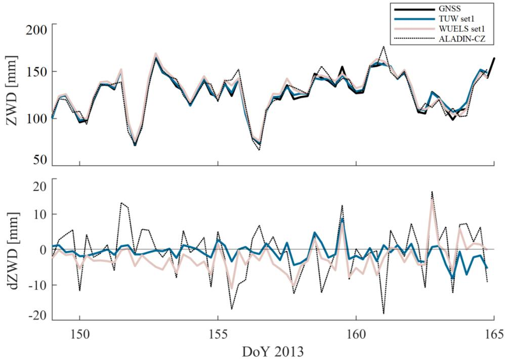
**Figure 4: GNSS-derived (black) and tomography-derived (blue and red) ZWD time series at GNSS site WTZR (Wetzell, Germany). The dashed line shows the ZWD values derived from the ALADIN-CZ model. The top plot shows the absolute values and the bottom plot highlights the ZWD differences with respect to the GNSS-derived ZWDs.**
