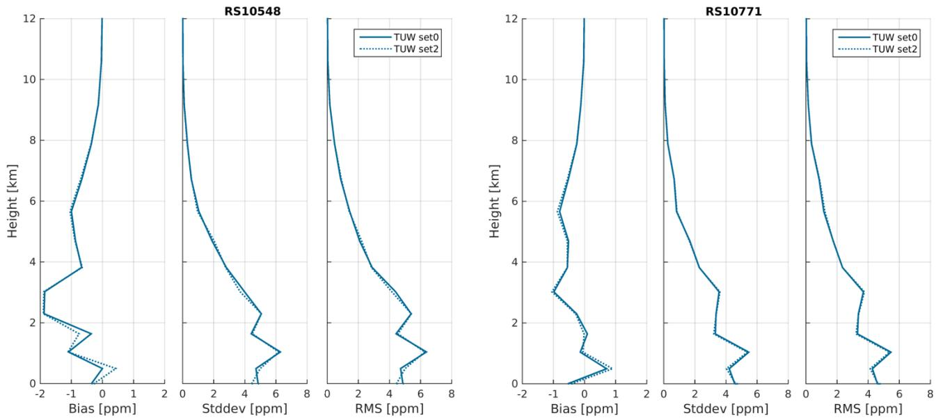
**Figure 7: Statistics of the differences in wet refractivity between radiosonde data and various tomography solutions. Differences between set0 and set2 are related to the strategy for compensation of the outer tropospheric delay.**
