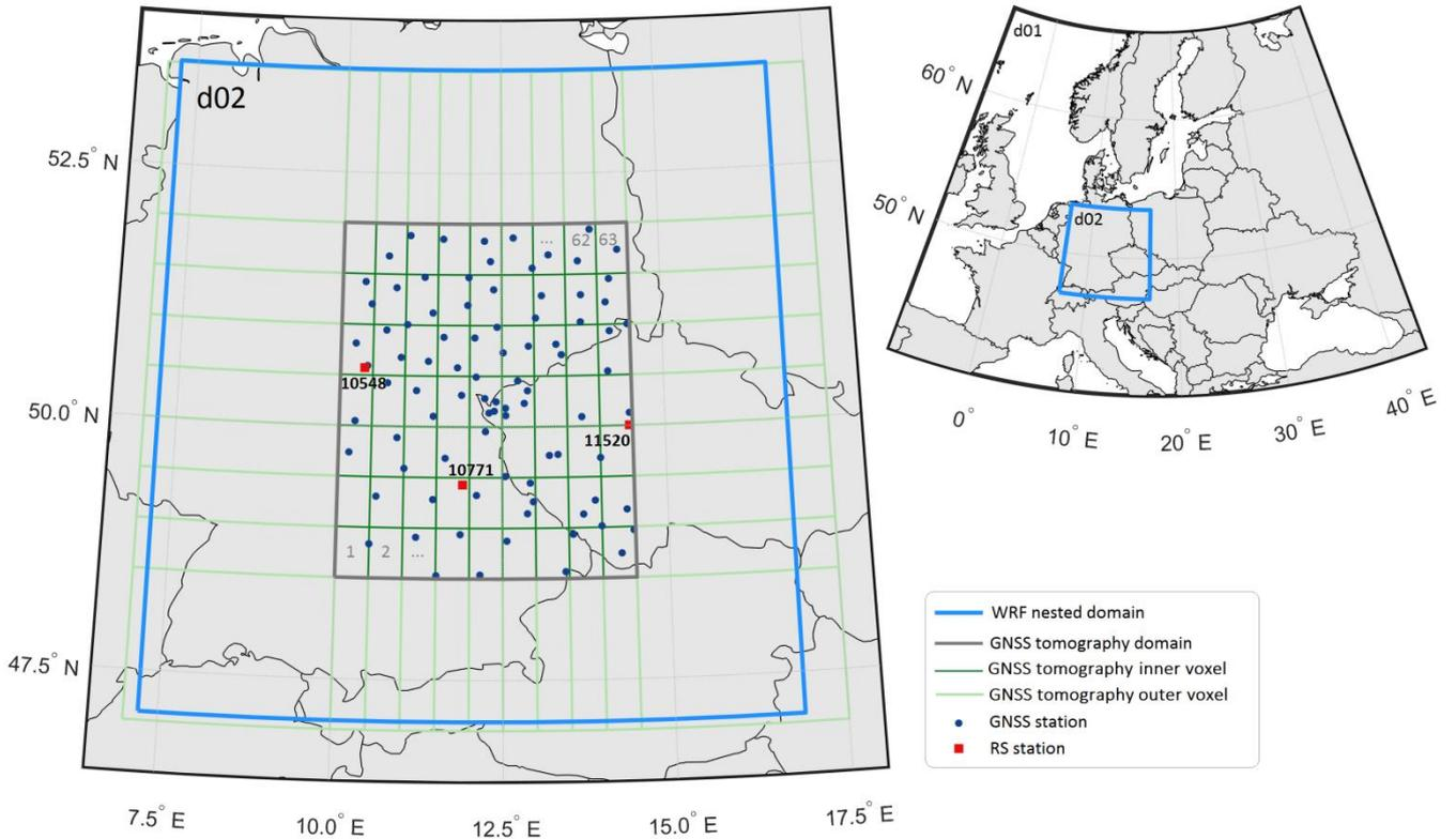
**Figure 2: The geographical extensions of the WRF domains used in this research (d01 = coarse grid with 36 km horizontal spacing, d02 = fine grid with 12 km horizontal spacing), GNSS tomography domain (grey line), together with inner (dark green line) and outer (light green line) voxels, including GNSS sites (dark blue dots) and radiosonde stations (red squares).**
