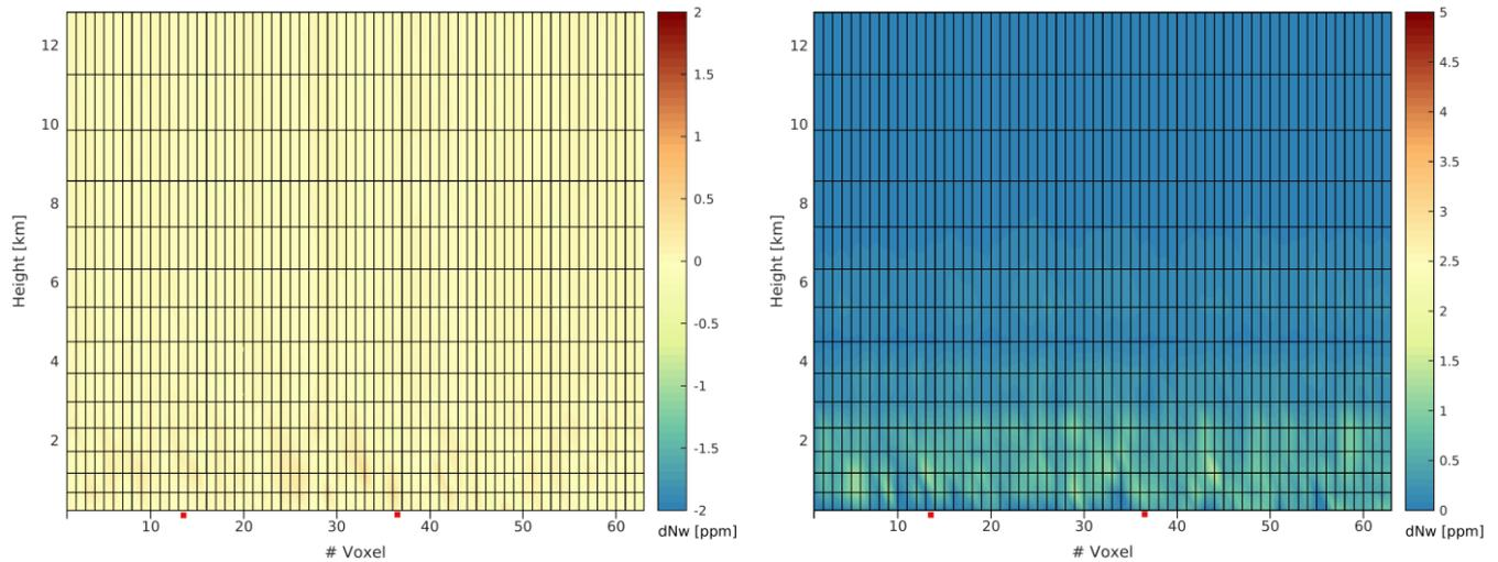
5 **Figure 3: Bias (left) and standard deviation (right) of the differences in wet refractivity [ppm] between TUV set0 and TUV set1. Analysed period: 29 May – 14 June 2013 (68 epochs). Red squares denote location of the RS stations.**
