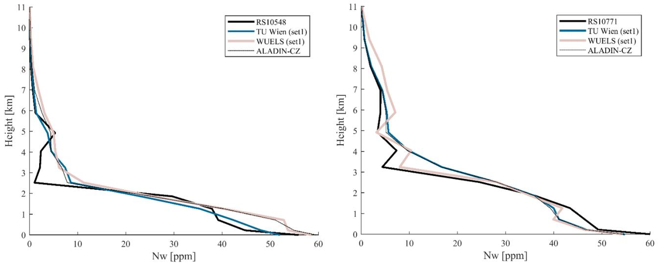
**Figure 5: Wet refractivity profiles derived from radiosonde launches, ALADIN-CZ 6-hour forecast data, TUW and WUELS tomography set1 for the 6<sup>th</sup> of June 2013, 12 UTC (left) and the 13<sup>th</sup> of June 2013, 00 UTC (right), respectively.**
