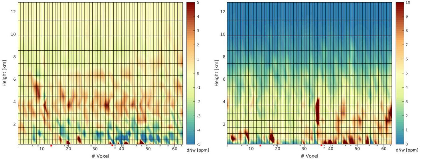
5 **Figure 5: Bias (left) and standard deviation (right) of the differences in wet refractivity [ppm] between TUV set1 and WUELS set1. Analysed period: 29 May – 14 June 2013 (68 epochs). Grey triangles denote GNSS stations removed from the specific voxels of the WUELS solution (one triangle stands for one rejected GNSS station), red squares denote location of the RS stations.**
