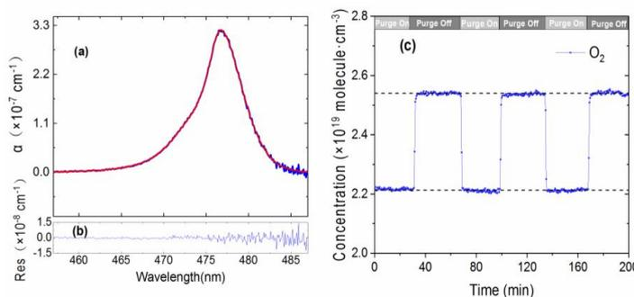
Fig. 3. (a) Example of retrieved and fitted absorption spectrum of O<sub>4</sub>. The blue line is the measured spectrum and the red line is the fitted spectrum of O<sub>4</sub>; (b) Fit residuals; (c) The time series of equivalent O<sub>2</sub> concentrations when N<sub>2</sub> purge gas was alternated between On and Off.
