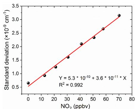
Fig. 9. The standard deviation of the fit residual from fig.7 as a function of  $\text{NO}_2$  concentrations.
