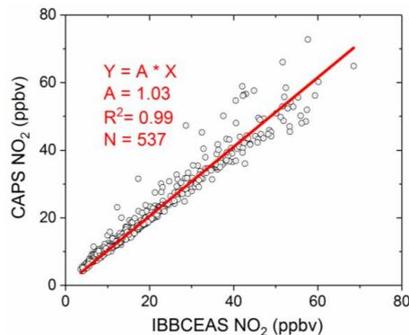
Fig. 14. Correlation plot of NO<sub>2</sub> concentration values between IBBCEAS and CAPS measurements. Each NO<sub>2</sub> data point was represented by averaged values to 1 h. The slope of the straight line fit (red line) is 1.03 with R<sup>2</sup> = 0.99
