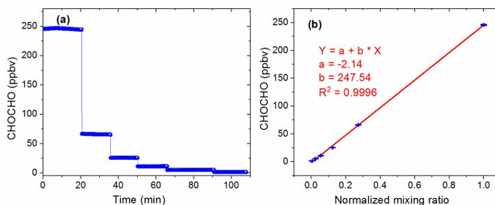
10 Fig. 6. Measurement of glyoxal sample gas. (a) Different concentrations of CHOCHO measured by IBBCEAS. (b) shows the correlation between the average of these concentration gradients and the normalized mixing ratio.
