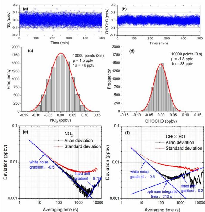
Fig. 4. Evaluation of the instrument performance. Panels (a) and (b) are the time series of NO<sub>2</sub> and CHOCHO with 3 s acquisition time. Panels (c) and (d) show the histogram analyses of the measurements of NO<sub>2</sub> and CHOCHO, respectively. Panels (e) and (f) are Allan deviation plots for measurements of NO<sub>2</sub> and CHOCHO, respectively.
