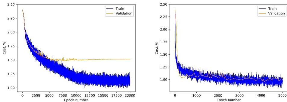
**Figure 109.** Siauliai ANN multi-species cost function for scatter (left) and fluorescence-(right) based recognition as a function of the training epoch.
