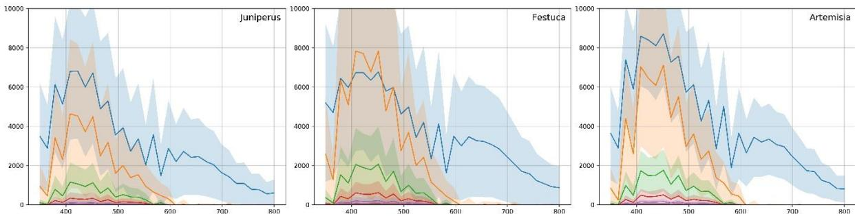
1420 **Figure 87.** Comparison of fluorescence indicators of the tested pollen. The blue line represents the first acquisition. All other lines are delayed acquisition by step of 500 ns from the last. Shadows show the standard deviation ranges for each acquisition. In the figures, the x-axis represents the wavelength, nm; the y axis shows the amplitude, NA
