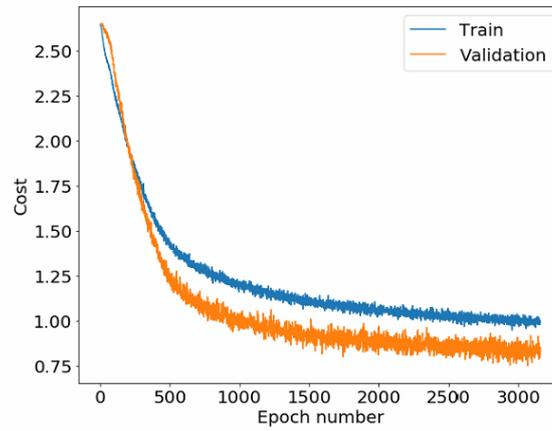
1435 **Figure 1110.** Novi Sad ANN overall cost as a function of the training epoch. The evaluation error is lower than the training error due to dropout (0.5) in each convolutional and fully connected layer, not used in the validation round.
