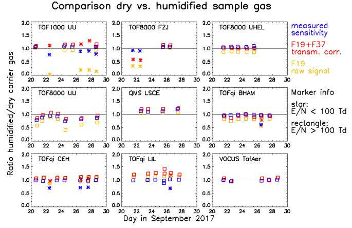
*Figure 8.* Comparison of gas standard injections using humidified and dry carrier gas. The ratios obtained for humidified versus dry injections are shown for (i) the mean measured sensitivity of a core set of compounds (blue), (ii) the transmission corrected primary ion signal (red), and (iii) the raw  $H_3O^+$  signal (yellow). The symbols separate measurements done at *E/N* levels above (rectangles) or below (stars) 100 Td.
