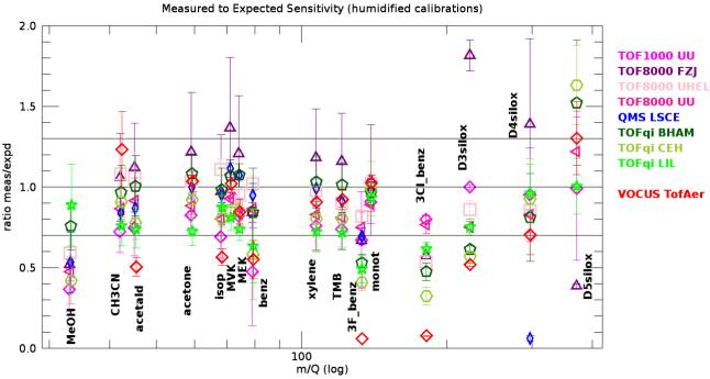
*Figure 7.* Measured versus expected sensitivities retrieved from humidified injections for all compounds in the gas standard and all PTR-MS instruments. The error bars represent the standard deviation of all gas standard injections with humidified  $N_2$  or air as carrier gas. Compounds as in Figure 4.
