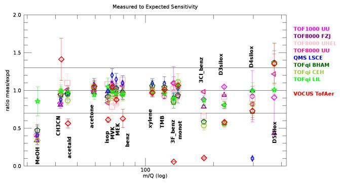
*Figure 5.* The ratio between measured and expected sensitivities as retrieved from dry injections that were not used for transmission retrievals. The data for most compounds and most instruments are well within +/-30%. The error bars represent the standard deviation of all gas standard injections with dry N<sub>2</sub> or air as carrier gas, except those that were used to calculate
