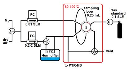
**Figure 1:** Schematic of the semi-automated calibration unit. Manual 3-way valves allow selection of dry air or nitrogen as carrier gas (valve 1), dry or humidified carrier gas (valve 2), and sample loop injections or dynamic mixing of carrier gas and gas standard (valve 3). Valve 4 (PFA-solenoid) and valve 5 (Valco 6-port with Restek sulfinert coating) are controlled to provide a sequence of 10 injections in one minute.
