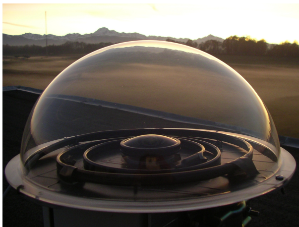
Figure 1. The RAPACE sky imager system developed at P2OA instrumented site. We can see the fish-eye at the center, the Plexiglas dome and the thermostatted heating wire in spiral around the fish eye.
