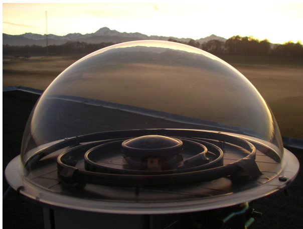
Figure 1. The RAPACE sky imager system developed at P2OA instrumented site. We can see the fisheye-lens at the center, the Plexiglas dome and the thermostatted heating wire in spiral around the fisheye.
