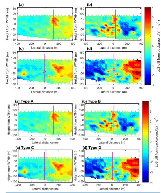
Figure 12. Representative examples of radial velocity anomalies at 2.5 D distance from the wind turbine for the four ease-types. The scanning Doppler lidar measurements are shown are individual points whereas the solid colours are cubic spline interpolated values. The results of the automated wake detection algorithm are shown as magenta circle for the wake centre. To aid visibility the location of the wake centre is extended vertically as a magenta line. The wake ease-types are;
