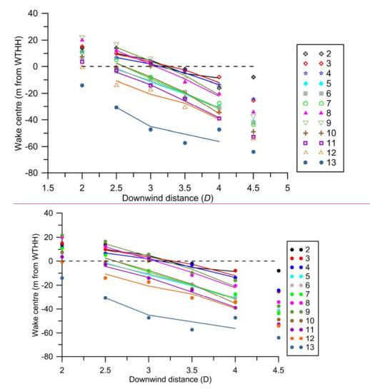
5 Figure 17. Mean vertical location of the wake centre conditionally sampled by inflow tower wind speed at 78 m height (in ms<sup>-1</sup>) for different distances downstream of the wind turbine location (A eases-type only).
