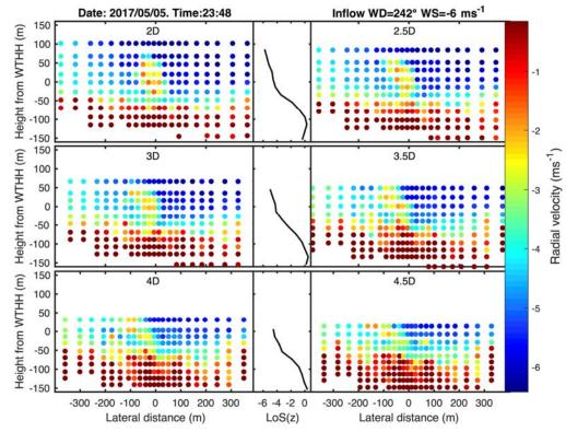
Figure 6. Example of raw radial wind speeds on planes at the six downstream distances 2, 2.5, 3, 3.5, 4 and 4.5 *D* from the arc scans on May 5 2017 at 23:48 (UTC) (shown in Figure 5). The middle three panels show the mean background radial wind speed profile (LoS(z)) at 2.5, 3.5 and 4.5 *D*. A lateral distance of 0 (on the x-axis) indicates a direct line to the wind turbine (i.e. a direction of 227°). The heights on the vertical axis have been normalized to be 0 at the *WTHH*.
