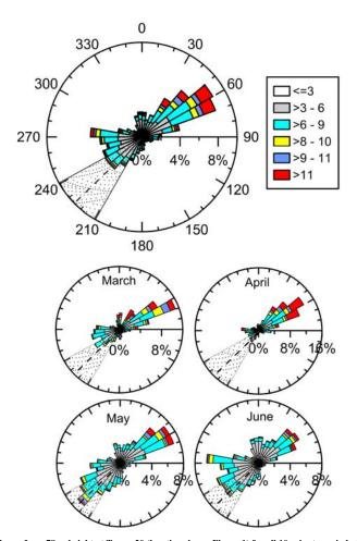
Figure 8. Top: Wind rose from 78 m height at Tower 20 (location shown Figure 1) for all 10-minute periods during March-June 2017. Coloured bars show the wind speed in ms<sup>-1</sup>. Below: Wind rose for each month. The shaded grey area shows the primary wake directions (209-241°) with the wake centreline direction of 227° marked with the black dashed line.
