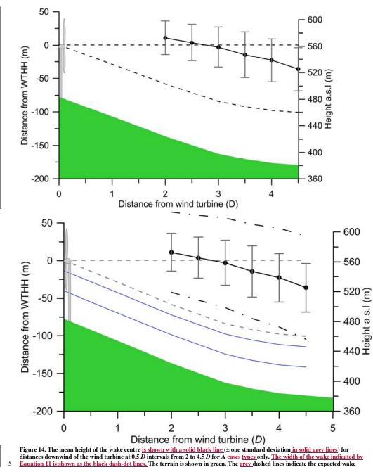
centre if it remained at the WTHH and for the case if where the centre is purely terrain-following. The solid blue lines indicate the range of heights for the inner layer from Table 1.
