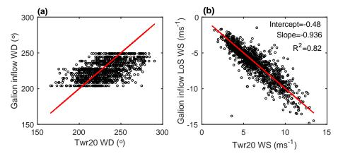
Figure 3. Comparison of 10-minute (a) inflow wind direction and (b) inflow wind speed at 78 m height from scanning Doppler lidar measurements (labelled Galion inflow) and those from the sonic anemometer deployed at 78 m on Tower 20 (shown as Twr20). Note the wind speeds reported by the Galion are radial line of sight velocities and are negative for flow towards the wind turbine. 1:1 lines are shown in red while each dot represents a 10-minute period (n = 1123).
