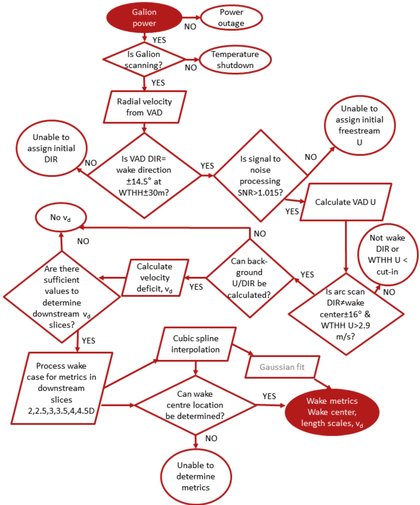
Figure 4. Flow chart outlining the automated wake processing of the Doppler lidar data for wake detection and characterization. The following abbreviations are used DIR=direction, U=wind speed, VAD DIR=direction retrieved from VAD scans, arc scan DIR=direction retrieved from arc scans. The Gaussian fit is not used here and hence is shown in grey.
