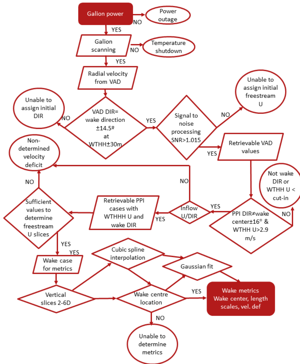
Figure 4. Flow chart outlining the automated wake processing of the Doppler lidar data for wake detection and characterization.
