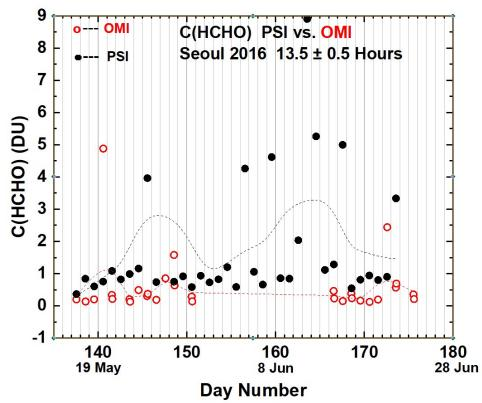
Fig. 21 Compare PSI ● and OMI o retrievals of C(HCHO) at 13.5 ± 0.5 hours. OMI overpass data, V03, are from https://avdc.gsfc.nasa.gov/index.php?site=1113974256&id=81
