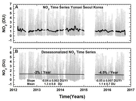
Fig. 7 (A)  $NO_2$  time series at Yonsei University in Seoul  $NO_2$ (grey) and (B) deseasonalized time series. Combined slope =  $-0.05 \pm 0.001$  DU/Year and Mean =  $1.2 \pm 0.8$  DU or the decrease is  $-4 \pm 0.08$  % / Year. Seoul has no clear seasonal cycle.
