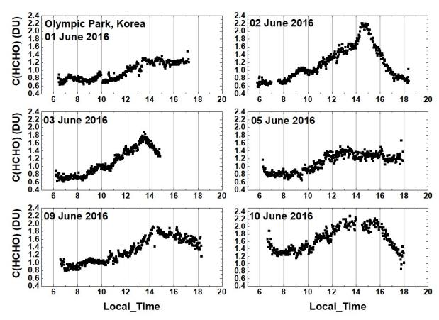
Fig. 12 C(HCHO) from PSI at Olympic Park for 6 days in June 2016. C(HCHO) on 2 June 2016 has a peak value of 2.3 DU at 14:30 hours.
