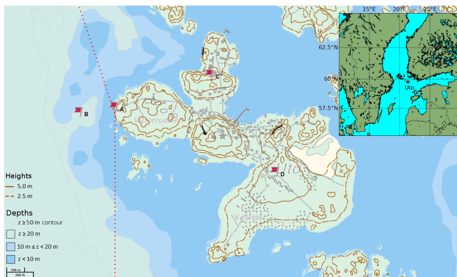
Figure 1. Location of the Utö island in the Archipelago Sea. The research installations on the island consist of the Utö Atmospheric and Marine Research Station (A), a flow-through pumping system (inlet at B), the Atmospheric ICOS station (C), and a weather and air quality station (D). The red dashed lines indicate the wind sector suitable for sea-air flux measurements (180–340°).
