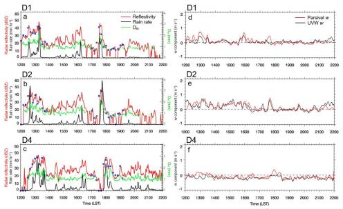
Figure 5. Time series of radar reflectivity (dBZ) in red line, rain rate (mm hr 1) in black, and massweighted mean diameter (D<sub>m</sub>, mm) in green at D1, D2, and D4 (left panels) and the time comparison of  $w_{par}$  (m s<sup>-1</sup>) in red and  $w_{UVW}$  (m s<sup>-1</sup>) in black at the same stations (right panels). Blue circles in the left panels indicate composite reflectivities (dBZ) from dual radars at the locations of D1, D2, and D4 for the selected periods.
