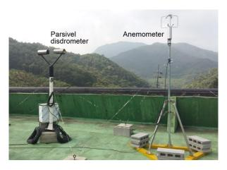
Figure 1. Picture of a Parsivel disdrometer and 3-D anemometer that were installed at a station around Mt. Jiri during the intensive observation period.
