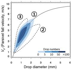
Figure 3. Schematic of Parsivel-observed diameter and fall velocity distributions for the three cases of determining zero w, upward w, and downward w. Contours show drop number concentrations. See text for more information.
