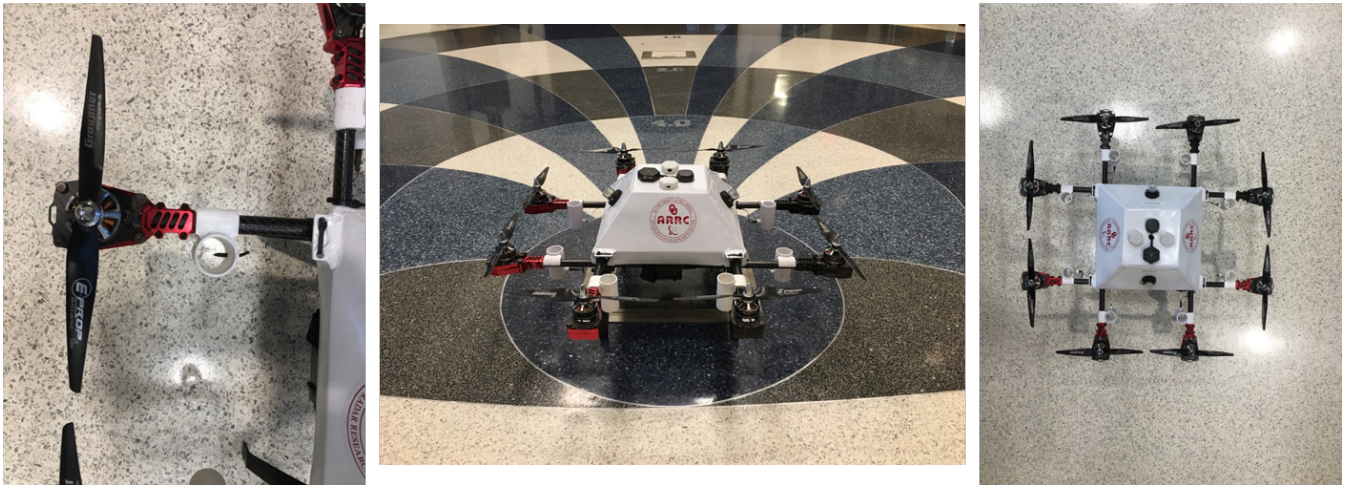
Figure 1. The CopterSonde, an octo-rotor UAS designed and built by the Center for Autonomous Sensing and Sampling at the University of Oklahoma.
