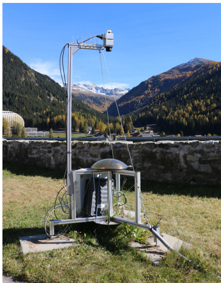
Figure 1. The Infrared Cloud Camera (IRCCAM) in the measurement enclosure of PMOD/WRC in Davos, Switzerland.
