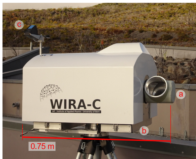
Figure 1. The WIRA-C instrument as installed on the Maïdo observatory on La Réunion island. It measures 0.6 \times 0.75 \times 0.5 m and contains the optics, the receiver, a spectrometer, a computer and power supplies. Radiation from the sky enters the instrument through the scan drum (a) which is at the same time the air outlet. Below the instrument, the air filters (b) are placed and on top, the GNSS antenna and a rain sensor (c) are attached.
