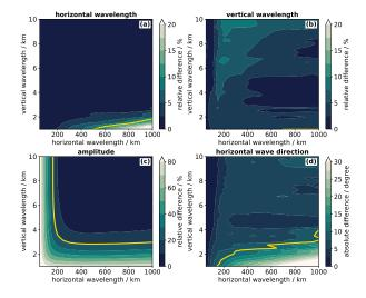
Figure 6. Specific observational filters for (a) horizontal wavelength  $\lambda_h$ , (b) vertical wavelength  $\lambda_z$ , (c) temperature amplitude  $\hat{T}$ , and (d) horizontal wave direction  $\varphi$  for the LAT retrieval and true horizontal wave orientation  $\varphi_t = 180^\circ$  and, thus, these waves have wavefronts perpendicular to the flight path. The yellow lines mark errors of 10%, 10%, 20% and 10° in Panels (a-d), respectively.
