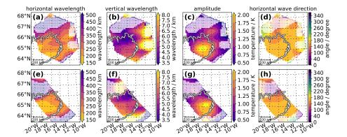
Figure 12. Wave parameters as obtained from the S3D fit with fitting cubes of  $160 \,\mathrm{km} \,\mathrm{x}\, 3.6 \,\mathrm{km}\, \mathrm{at}$  center height of  $11.5 \,\mathrm{km}$  for FAT (a-d) and LAT (e-h). Nonsignificant fitting results with wavelengths above 2.5 times the cube size are shaded. Panel (a) to (d) are adapted from Krisch et al. (2017) Fig. 5.
