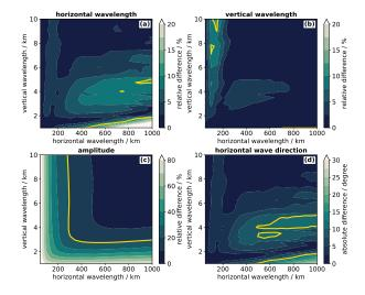
Figure 8. Specific observational filters for (a) horizontal wavelength  $\lambda_h$ , (b) vertical wavelength  $\lambda_z$ , (c) temperature amplitude  $\hat{T}$ , and (d) horizontal wave direction  $\varphi$  for the LAT retrieval with true horizontal wave orientation  $\varphi_t = 210^\circ$  and, thus, waves, which are tilted towards the aircraft. The yellow lines mark errors of 10%, 10%, 20% and  $10^\circ$  in Panels (a-d), respectively.
