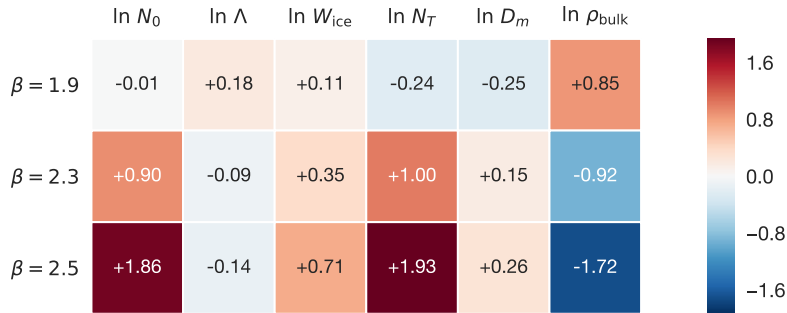
Figure 7. The root-mean-square changes in the microphysical parameters in response to changes in the mass–dimensional exponent \beta . The standard assumption of this paper, \beta = 2.1 , is used as the baseline. The value of \beta is indicated on the left side of each row. The analysis is based on the December 4, 2015, case (Sect. 5.2).
