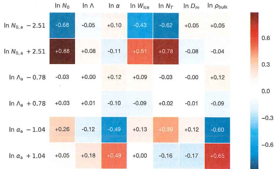
Figure 6. The root-mean-square changes in the microphysical parameters in response to changes in the prior. The change in the prior is indicated on the left side of each row. The data are from the December 4, 2015, case (Sect. 5.2).
