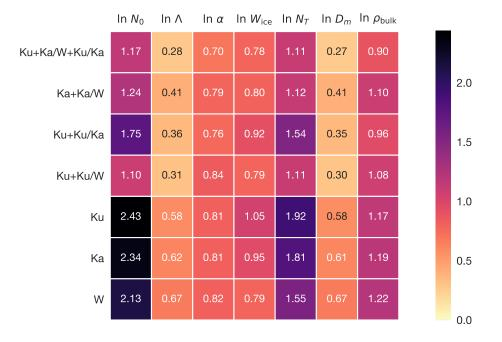
**Figure 5.** The average posterior retrieval errors of the logarithms of microphysical variables with different combinations of radar frequencies. The data from the December 4, 2015, case (Sect. 5.2) is used in this figure.
