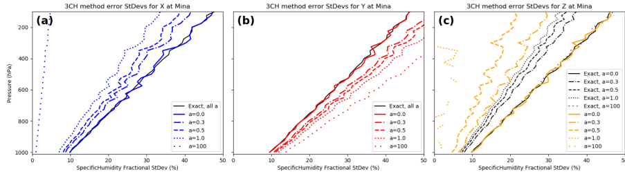
Figure 3. (a) Estimated standard deviation of X_{\text{err}} for values of a = 0, 0.3, 0.5, 1.0 and 100 computed from Eq. (3a)–(5a). Exact STD computed from data set X (solid black profile). (b) Same as (a) except for estimated STD of Y_{\text{err}} . (c) Same as (a) except for estimated STD of Z_{\text{err}} . Note that for different values of a , the exact STD of X_{\text{err}} and Y_{\text{err}} are always the same. The exact STD of decreases Z_{\text{err}} as a increases for 0 < a < 1.0 . For a > 1.0 , the exact STD of Z_{\text{err}} increases as a increases, becoming equal to the STD of X_{\text{err}} for a = \infty due to the way our error model is defined (see also Table 1). For a = 100 the correlation between X and Z errors is 0.99995 (Table 1; black dotted line for a = 100 almost identical to black solid line for a = 0 ).
