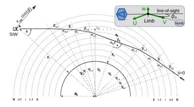
**Figure 4.** Limb sounding geometry for a refracted line-of-sight (full line) and a none refracted one (dashed line). The panel on the right-upper corner shows the orientation of the LOS with respect to the wind components at the tangent point. Figure is adapted from Urban et al. (2004).
