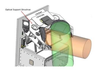
**Figure 1.** View of the Innosat satellite. The box in the lower-part is the platform service module. Above it is the scientific payload including the two antennas. The field of views are represented with green and beige colors (from Omnisys instruments co).
