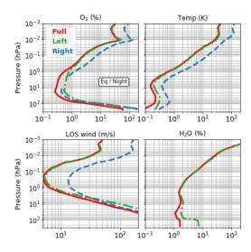
Figure 8. Single-scan retrieval precision  $(1-\sigma)$  for  $O_3$  and temperature (upper panels), and line-of-sight wind and  $H_2O$  (lower panels). Errors are calculated for a full band retrieval (red lines), the left half IF-band (10.075-14.075 GHz), blue lines) and the right half IF band (14.075-18.075 GHz), green lines). Results are shown for Equatorial nighttime conditions.
