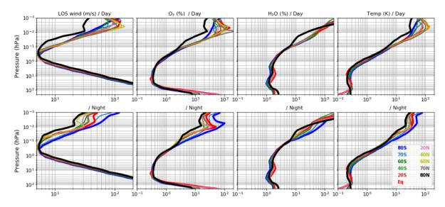
Figure 7. Single-scan retrieval precision  $(1-\sigma)$  for line-of-sight wind (left-most panels),  $O_3$  (2nd column panels),  $H_2O$  (3rd column panels), and temperature (right-most panels). The line colors correspond to latitude bins (see legend) and thick lines are used for those corresponding to polar and equatorial regions. Errors are given for day- and nighttime labeled profiles. Note that southern (northern) polar profiles are actually both daytime (nighttime) ones.
