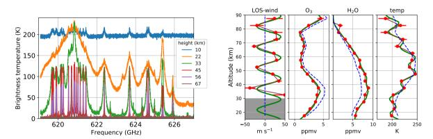
**Figure 6.** Left panel: Double sideband spectra with respect to the lower sideband frequency. Only a few spectra of the full vertical scan are shown (see legend). Right panel: Retrieved profiles with a vertical resolution of 5 km for nighttime arctic conditions. The blue-dashed lines are the a priori profiles (first guess), the green lines are the truth and the red line-circles are the retrieved values. The horizontal bars indicate the  $1-\sigma$  errors due to instrument thermal noise.
