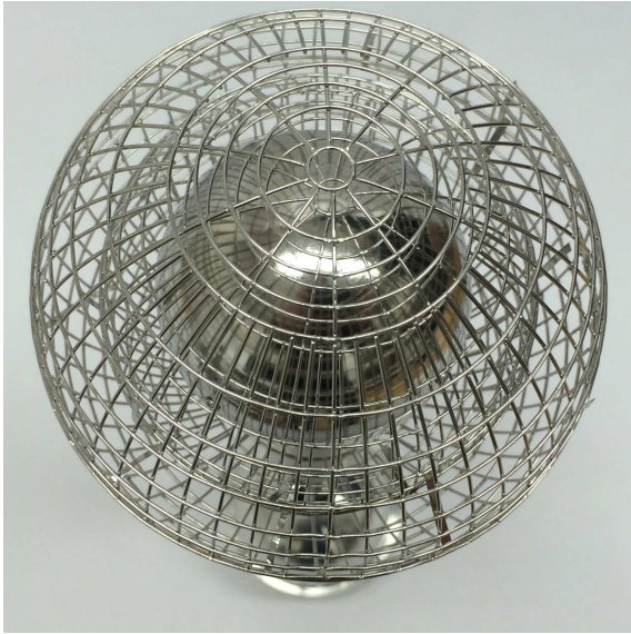
Figure 1. Meteor Smoke Particle Detector with its central spherical electrode (26 mm radius) shielded by two electrically biased concentric grids (35 mm and 45 mm radius).
