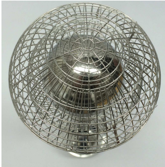
Figure 1. Meteoric Smoke Particle Detector with its central spherical electrode (26 mm radius) shielded by two electrically biased concentric grids (35 mm and 45 mm radius).
