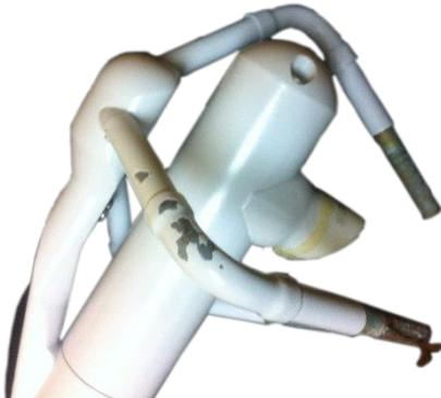
Figure 3: Painting off as apparently impacted on the knuckle of side claw (i.e., ~~1<sup>st</sup>~~ first sonic path) among the top three sonic transducer claws of IRGASON sonic anemometer.
