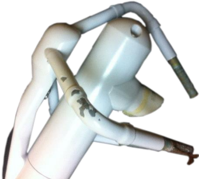
Figure 3: Painting off as apparently impacted on the knuckle of side claw (first sonic path) among the top three sonic transducer claws of IRGASON sonic anemometer (Serial Number: 1131).
