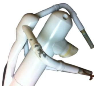
Figure 3: Painting off as apparently impacted on the knuckle of side claw (i.e., 1<sup>st</sup> sonic path) among the top three sonic transducer claws of IRGASON sonic anemometer.
