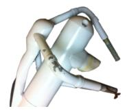
Figure 3: Painting off as apparently impacted on the knuckle of side claw (i.e., 1<sup>st</sup> sonic path) among the top three sonic transducer claws of IRGASON sonic anemometer.
