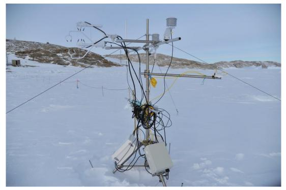
Figure 2: The eddy-covariance station located in the coastal landfast sea ice area of Antarctica Zhongshan Station (69°22' S, 76°22' E). It was configured with IRGASON integrated CO<sub>2</sub>/H<sub>2</sub>O open-path gas analyzer and three-dimensional sonic anemometer, CNR4 4-Way Net Radiometer, HMP155A air temperature and relative humidity probe, and SI-111 infrared radiometer.
