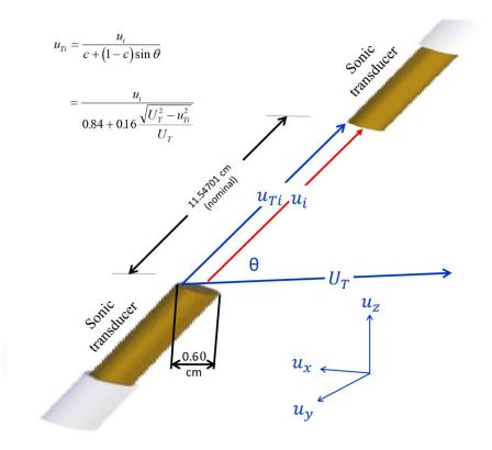
Figure 4: Sonic transducer shadowing [Along the *i*th (i = 1, 2, or 3) sonic path between the two sonic transducers,  $u_i$  is the measured magnitude of flow vector whose true magnitude is  $u_{Ti}$ ;  $u_{\perp i}$  is the flow speed normal to the *i*<sup>th</sup> sonic path;  $u_x, u_y$ , and  $u_z$  are the wind speeds expressed in the three-dimensional instrument coordinate system; and  $\alpha_i$  is the angle between sonic
