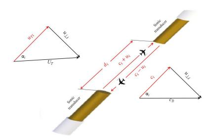
Figure 5: Crosswind on speed of sound. Along the *i*th (i = 1, 2, or 3) sonic path between the two sonic transducers,  $u_i$  is the measured magnitude of flow vector whose true magnitude is  $u_{Ti}$ , and  $c_i$  is measured speed of sound;  $u_{Li}$  is the crosswind vector
