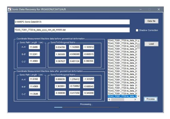
5 Figure 6: Dialogue interface of software: Sonic Data Recovery for IRGASON/CSAT3/A/B Used in Geometrical Deformation after Production/Calibration.
