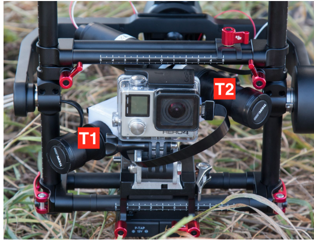
Figure 2. Gimbal payload: GoPro camera and two telescopes highlighted with T1 and T2 (here mounted with 90° opening angle between them) with protective lens caps. Picture taken from the photo gallery https://work.courtney.dk/#collection/7 .
