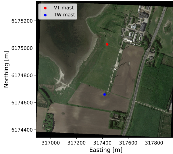
Figure 3. Aerial photo of test center at Risø campus: blue point - position of 10 m mast denoted 'TW', red point - position of 70 m mast denoted 'VT'. Aerial data: ©Google Maps, DigitalGlobe.
