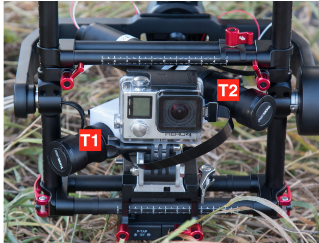
Figure 2. Gimbal payload: GoPro camera and two telescopes highlighted with T1 and T2 (here mounted with 90^\circ opening angle between them) with protective lens caps. Picture taken from the photo gallery https://work.courtney.dk/#collection/7 .
