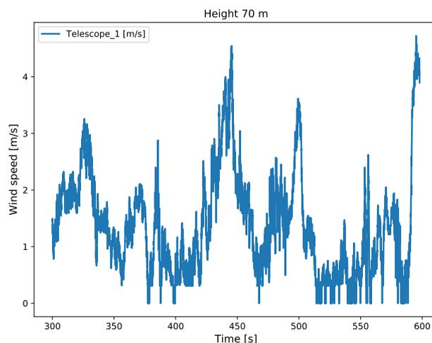
**Figure 4.** Time series showing measured LOS wind speed from preliminary drone-mounted lidar experiment
