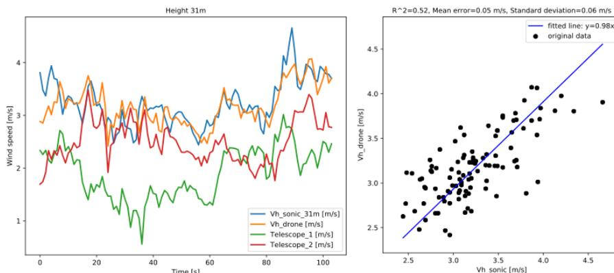
**Figure 12.** Comparison of measurements acquired at 31 m agl
