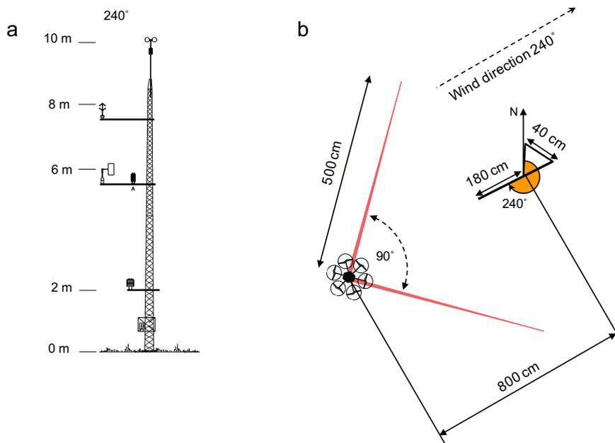
**Figure 7.** First experiment configuration: (a) 10-m mast sketch with position of instruments (2 m - humidity and temperature probe, 6 m - wind vane and humidity and temperature probe, 8 m - sonic anemometer, 10 m - cup anemometer); (b) 10-m mast cross section at 8 m height with the orientation of the drone with respect to the boom at which the sonic anemometer is installed.
