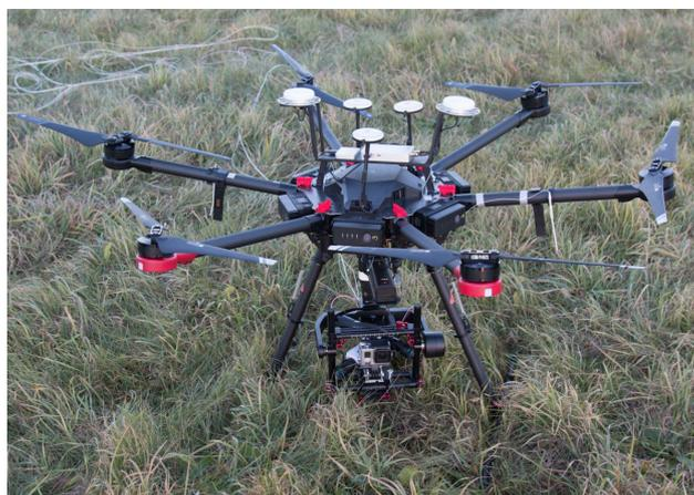
**Figure 2.** Complete system on ground: three central antennas - GNSS receivers for positioning, two side antennas - GNSS RTK receivers for real time position correction, white cable - four joined optical fibres. Picture taken from the photo gallery <https://work.courtney.dk/#collection/7>.
