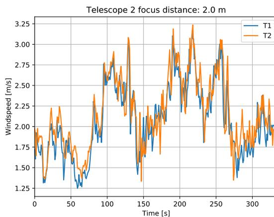
**Figure 17.** Example of 1-s averaged wind speed measurements acquired by the two telescopes with telescope 1 focused at 5 m and telescope 2 at 2 m.
