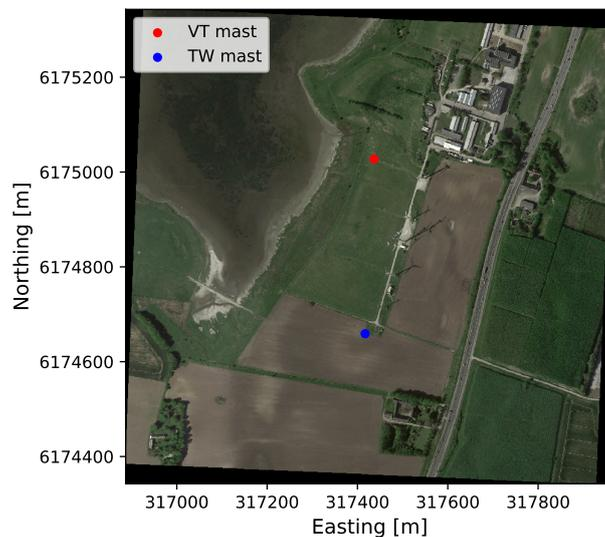
**Figure 5.** Aerial photo of test center at Risø campus: blue point - position of 10 m mast denoted 'TW', red point - position of 70 m mast denoted 'VT'. Aerial data: ©Google Maps, DigitalGlobe.
