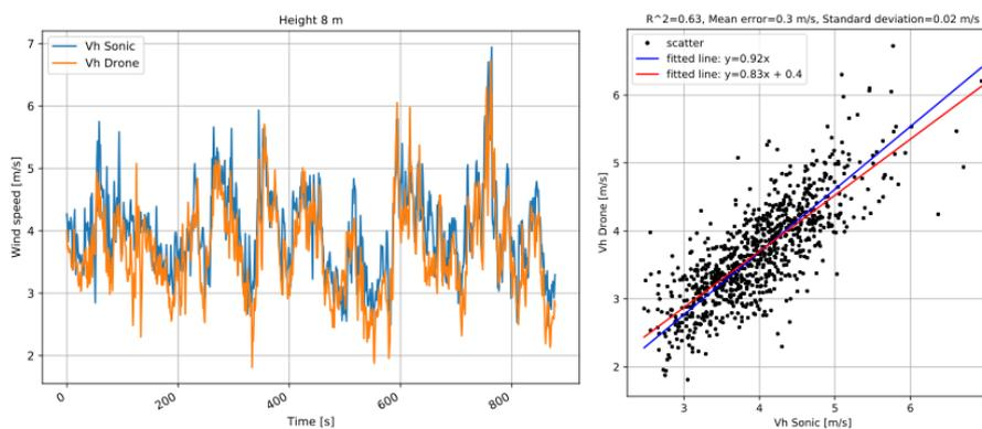
**Figure 8.** Measurements acquired next to the TW mast: left - 1 Hz time series of the horizontal wind speed acquired with the drone-lidar system and the sonic anemometer, right - linear regression plot.
