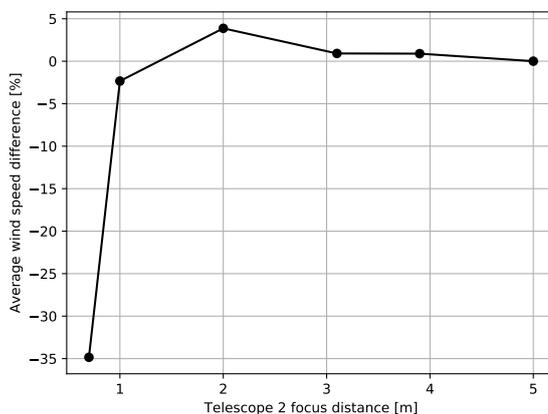
**Figure 19.** Relative difference in average wind speed measured by the two telescopes as function of telescope 2 focus distance.
