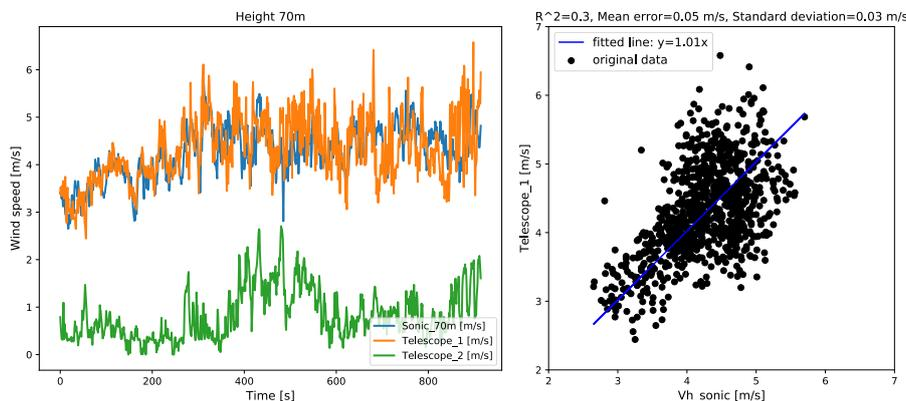
**Figure 16.** Single beam comparison at 70 m
