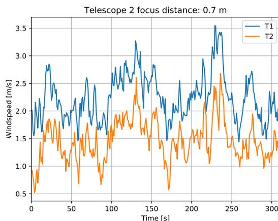
**Figure 18.** Example of 1-s averaged wind speed measurements acquired by the two telescopes with telescope 1 focused at 5 m and telescope 2 at 0.7 m. Clear differences are seen due to telescope 2 measuring inside the drone disturbance zone.
