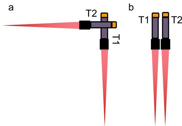
**Figure 6.** Telescope setup: a) opening angle of  $90^\circ$ , b) opening angle of  $0^\circ$
