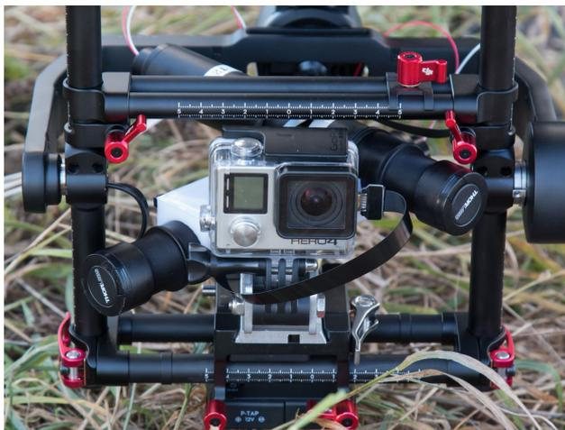
**Figure 3.** Gimbal payload: GoPro camera and two telescopes (here mounted with  $90^\circ$  opening angle between them) with protective lens caps. Picture taken from the photo gallery <https://work.courtney.dk/#collection/7>.
