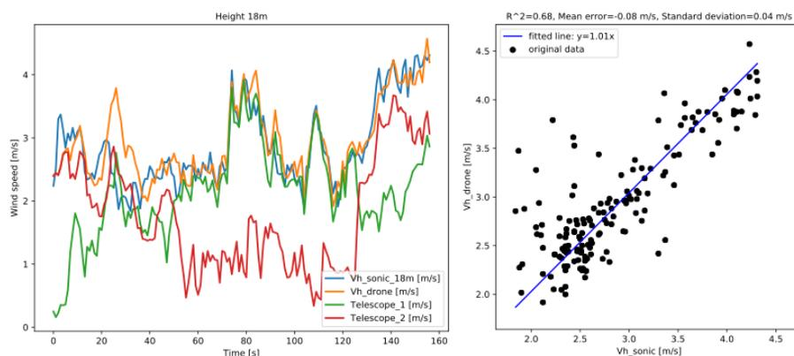
**Figure 11.** Comparison of measurements acquired at 18 m agl
