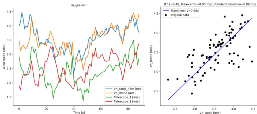
**Figure 13.** Comparison of measurements acquired at 44 m agl
