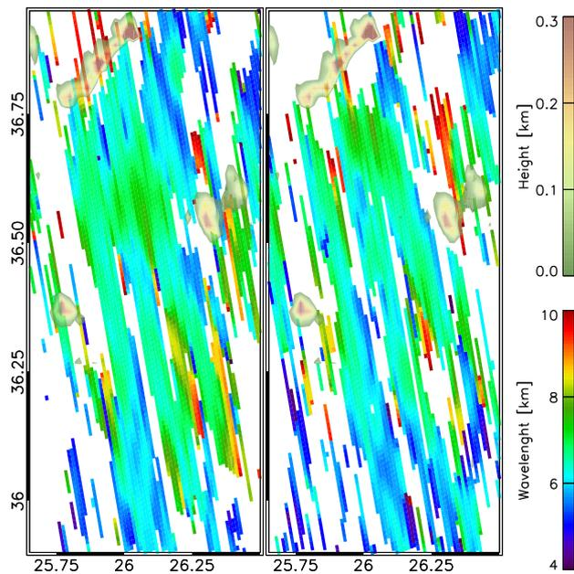
**Figure 6.** Wavelength, indicated by the lower bar with a colour scale ranging from 4 to 10 km, as derived applying the CWT method over the AIRWAVE TCWV products shown in Fig 4. The left panel shows ATSR-2 orbit 38086 (ascending), the right panel AATSR orbit 2214 (ascending). The height of the ground is also shown (upper bar).
