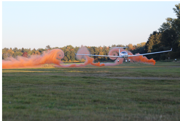
Figure 6. Illustration of small-scale concentration variability induced by aircraft. The photo was taken at the air field Aue/Hattorf, Germany, on 2 October 2011 at 16:15 UTC, copyright Institute of Flight Guidance, TU Braunschweig
