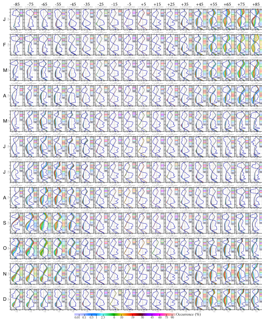
Figure 6. Climatological temperature profiles corresponding to the daytime M2TCO3 O_3 profiles shown in Fig. 3. The color scheme is the same as that in Fig. 3. The dashed dark blue line represents the coefficient of correlation between O_3 partial pressure and temperature as a function of pressure altitude Z^* .
