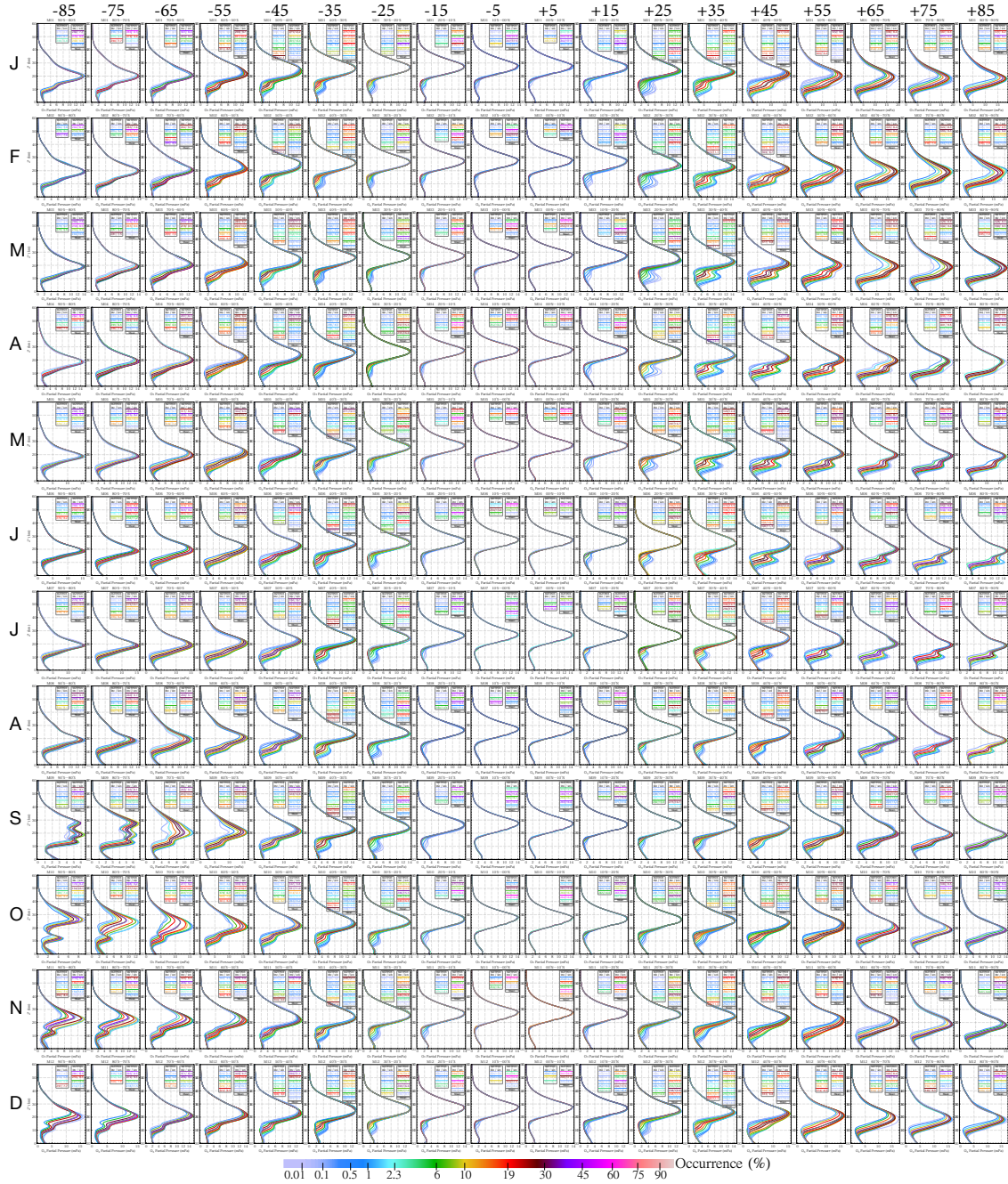
Figure 1. The daytime M2TPO3 climatology contains 2154 O 3 profiles that distribute among the 12×18 month-latitude classes. The color of a solid line indicates the percentage occurrence of the profile. The line legends display the average tropopause altitudes and the average total O 3 columns. The solid gray line represents the downgraded M2TPO3 profile, i.e., the monthly zonal mean profile.
