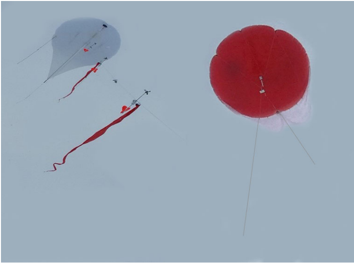
10 Figure 1. 34 m 3 helikite in flight with three tethersondes (left) and 79 m 3 aerostat in flight with radar calibration sphere (right).
