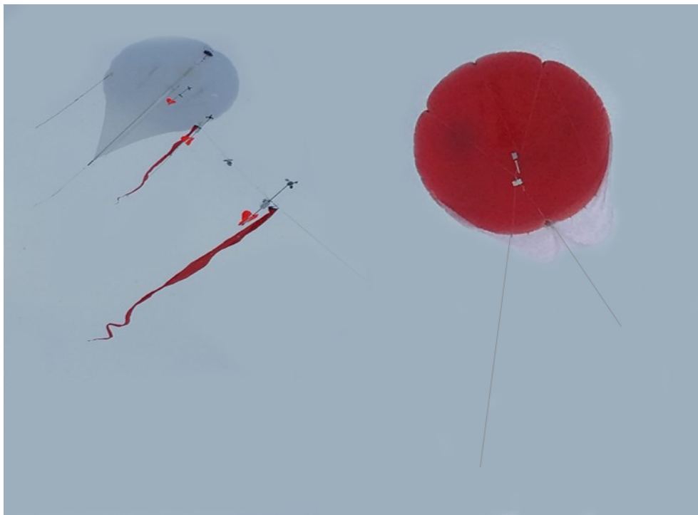
Figure 1. 34 \text{m}^3 helikite in flight with three tethersondes (left) and 79 \text{m}^3 aerostat in flight with radar calibration sphere (right).
