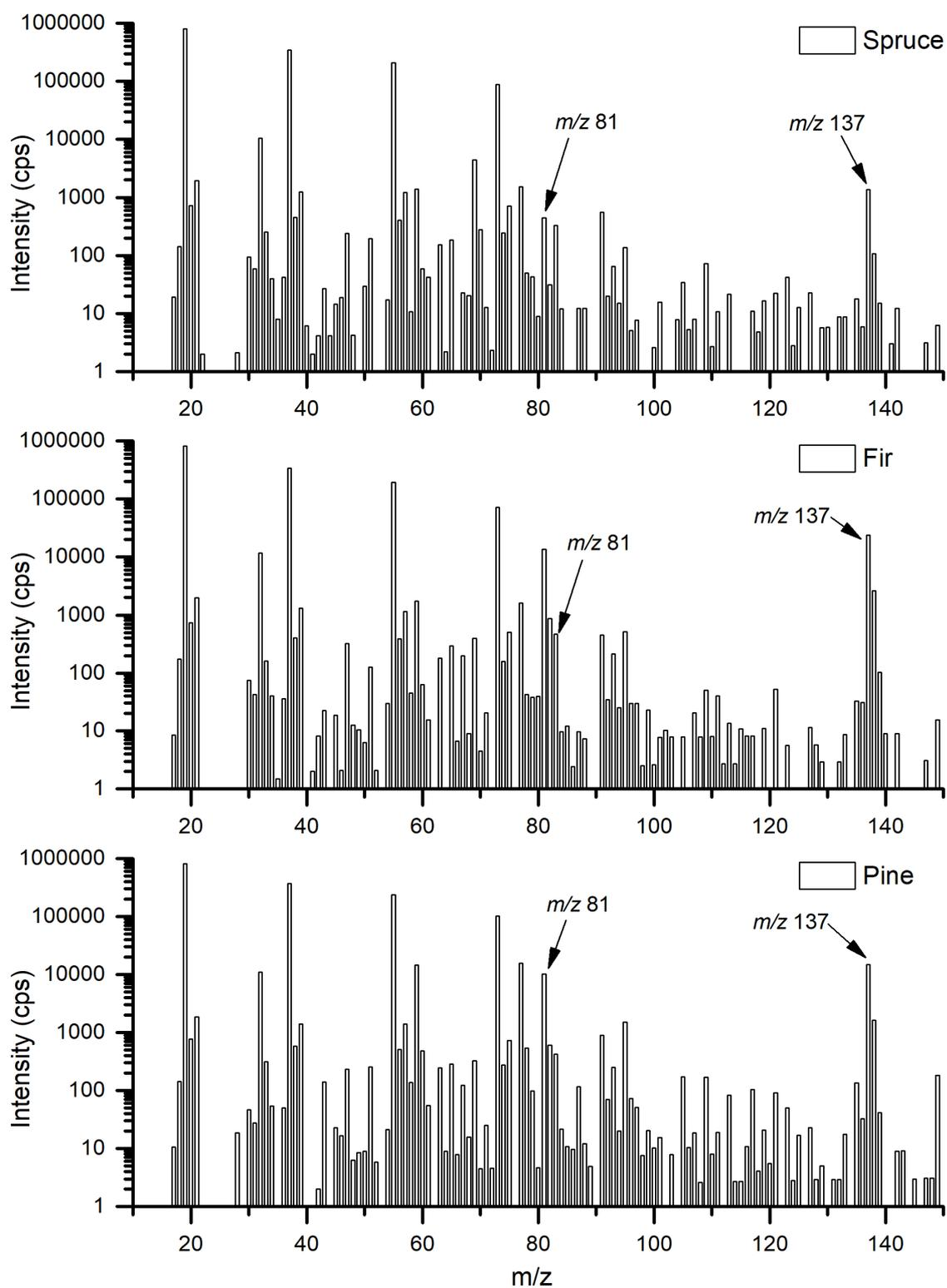
**Figure S3: SIFT-MS spectra of coniferous samples analysed by  $H_3O^+$  reagent ions. The marked ions with  $m/z$  81 and  $m/z$  137 were used for analysis of monoterpenes.**
