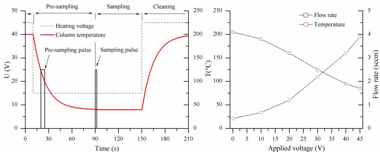
10 **Figure 2:** Left: the applied heating voltage (dashed) and the temperature profile of the column (red) during the fast GC cycle. The pulses indicate the opening of the valve EV3 during the pre-sampling and the sampling periods. Right: The increase of the column temperature and the related decrease of the carrier gas flow rate with the heating voltage.
