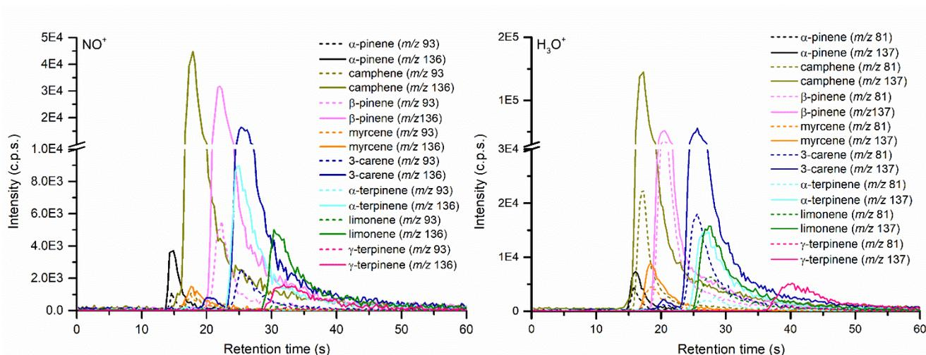
**Figure S2: Chromatograms of individual monoterpenes analysed using the MXT-1 column at a constant temperature of column ~40 °C. The profile is associated with the profile shown in the bottom of Figure S1. Profiles were analysed by SIFT-MS using the H<sub>3</sub>O<sup>+</sup> reagent ion. Intensity of  $\alpha$ -pinene was reduced.**
