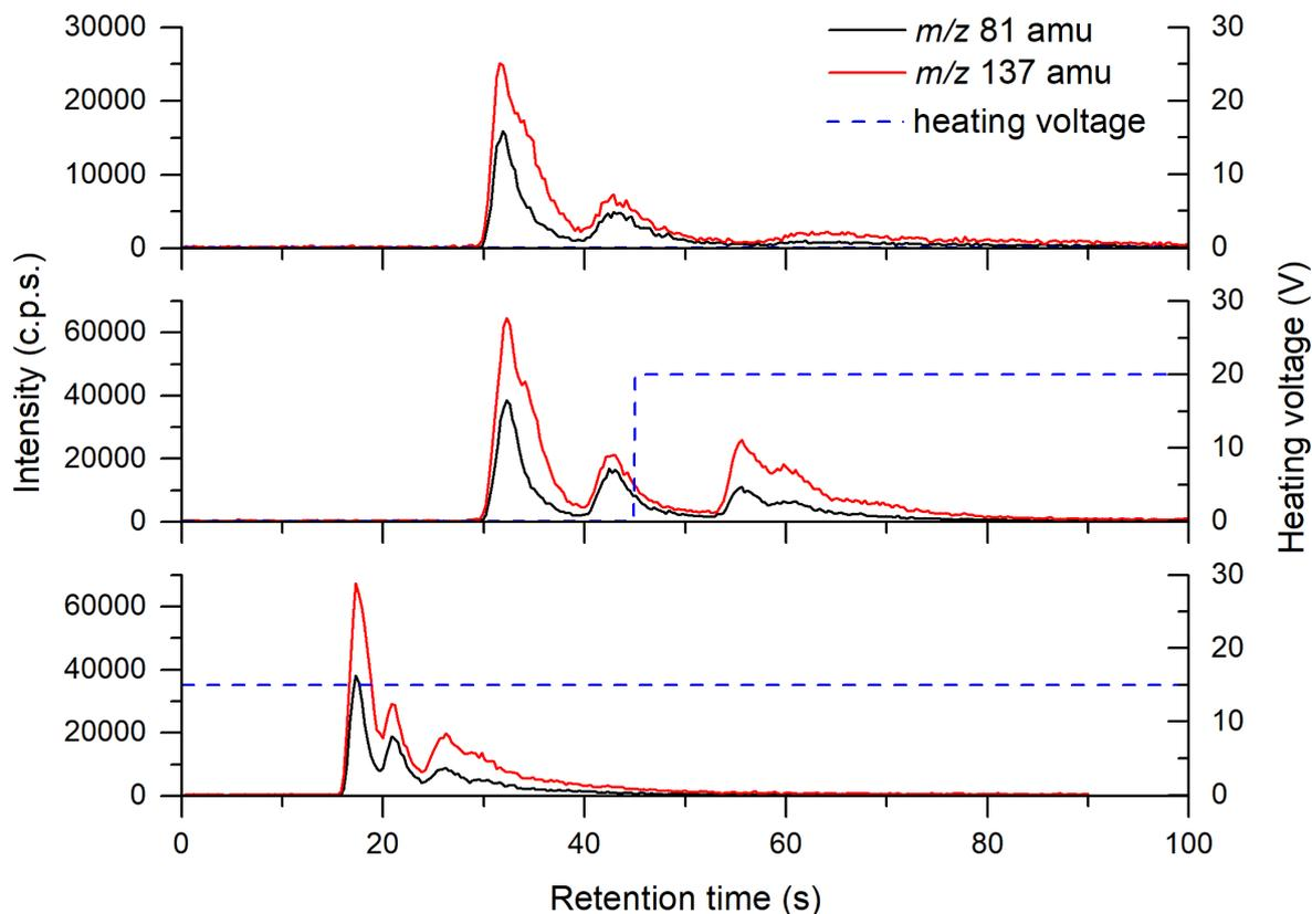
Figure S1: Chromatograms of a monoterpene mixture analysed by the MXT-1 column for different profiles of the heating voltage. Profiles were analysed by SIFT-MS using the  $\text{H}_3\text{O}^+$  reagent ion.
