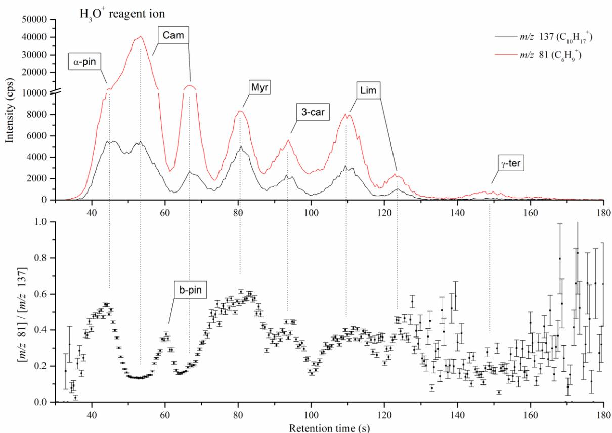
Figure 4: A chromatogram for a prepared mixture of monoterpenes obtained with the MXT-Volatiles column as derived by SIFT-MS using  $\text{H}_3\text{O}^+$  reagent ions. For the chromatogram, the product ion signal ratio  $r_i$  is presented in the bottom figure. This chromatogram was obtained at the column temperature  $\sim 45^\circ\text{C}$  using 20 V heating voltage (separation is faster compare to data on Table 1).
