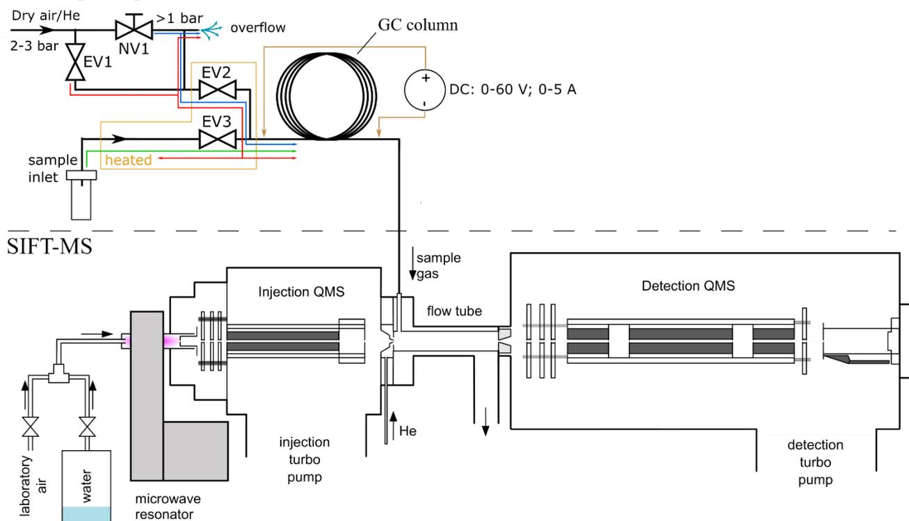
**Figure 1: Schematic visualization of the fast GC-SIFT-MS experiment. Coloured dashed lines in the inlet part of the ~~fastGC~~fast GC represent gas flow through the system of the valves EV1-3. The blue line traces the “normal mode” regime, the green line represents the “sampling mode” and the red line represents the “cleaning mode”.**
