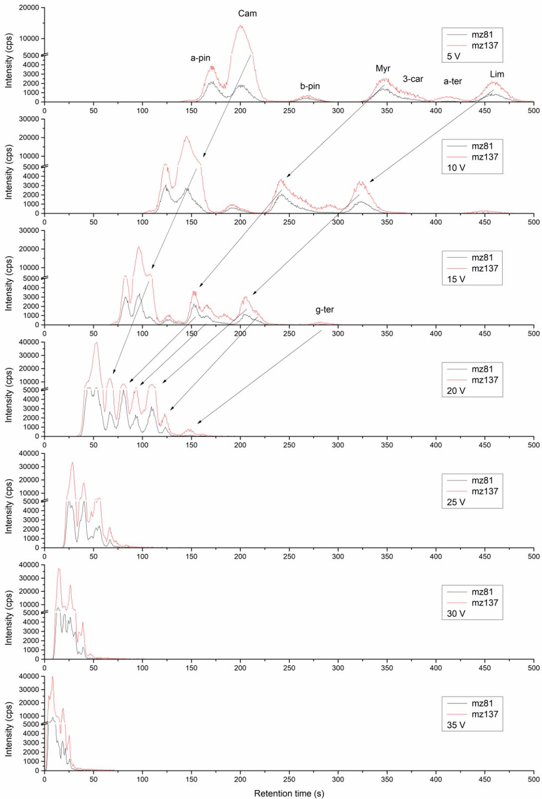
**Figure S4:** Chromatograms of a monoterpene mixture analysed by the MXT- Volatiles column for different heating voltages. Profiles were analysed by SIFT-MS using the  $\text{H}_3\text{O}^+$  reagent ion.
